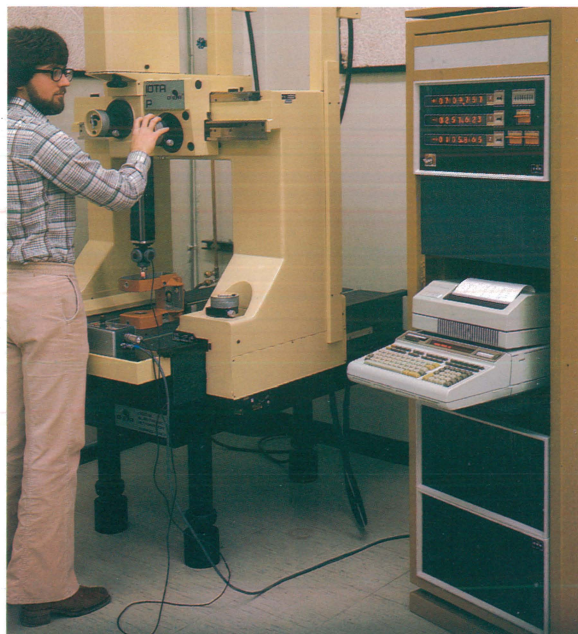
A 9825 guides the operator of a coordinate measuring machine through the inspection of a part. The 9825 records measurements, performs calculations and provides a finished report.
