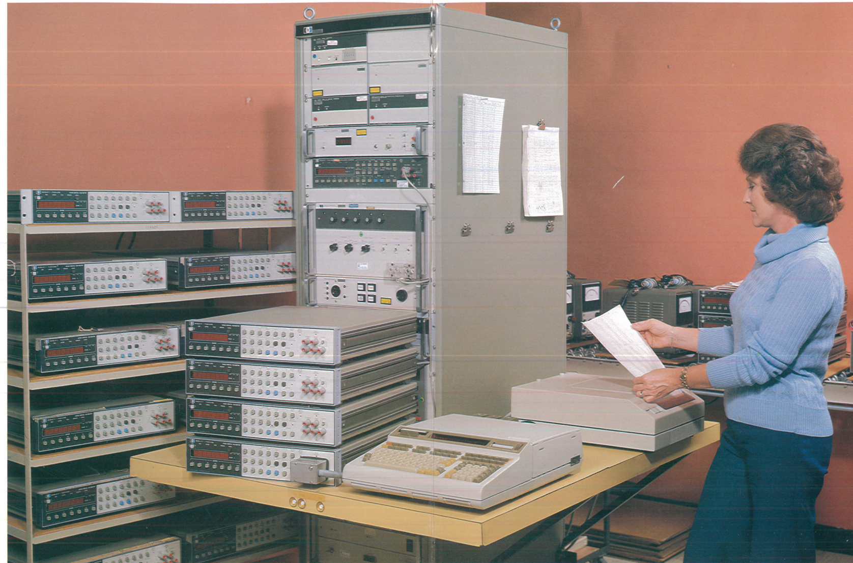
A 9825 controls the automated testing of digital voltmeters, acquires test data and prints out results on a peripheral printer.
