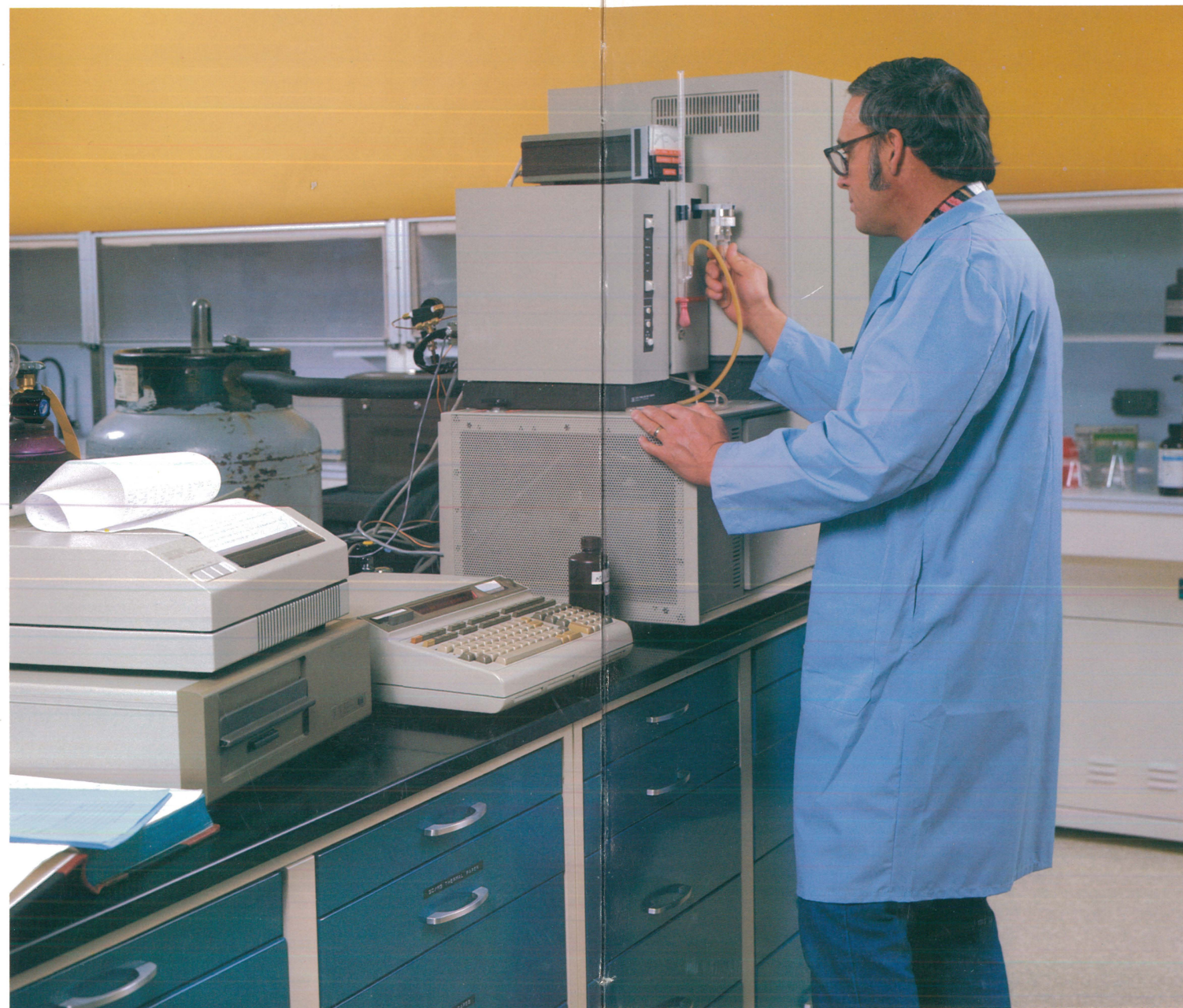
Many 9825s are employed in the physical and life sciences. Here, a 9825 analyzes data from a gas-chromatograph/mass-spectrometer system.
