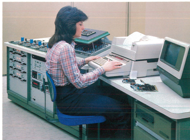
The 9825 is widely used for testing electronic circuits. It speeds up production economically.
