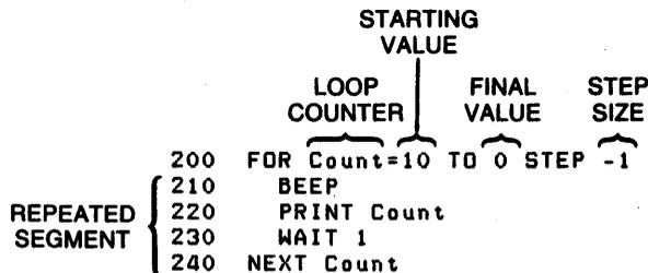
Figure 2-7. FOR...NEXT Loop Structure
