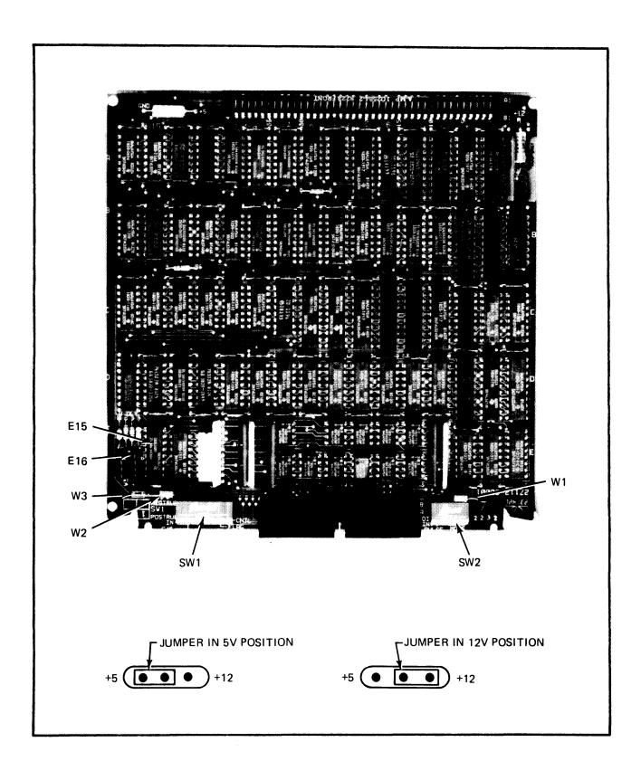
Figure 1. Switch and Jumper Locations
