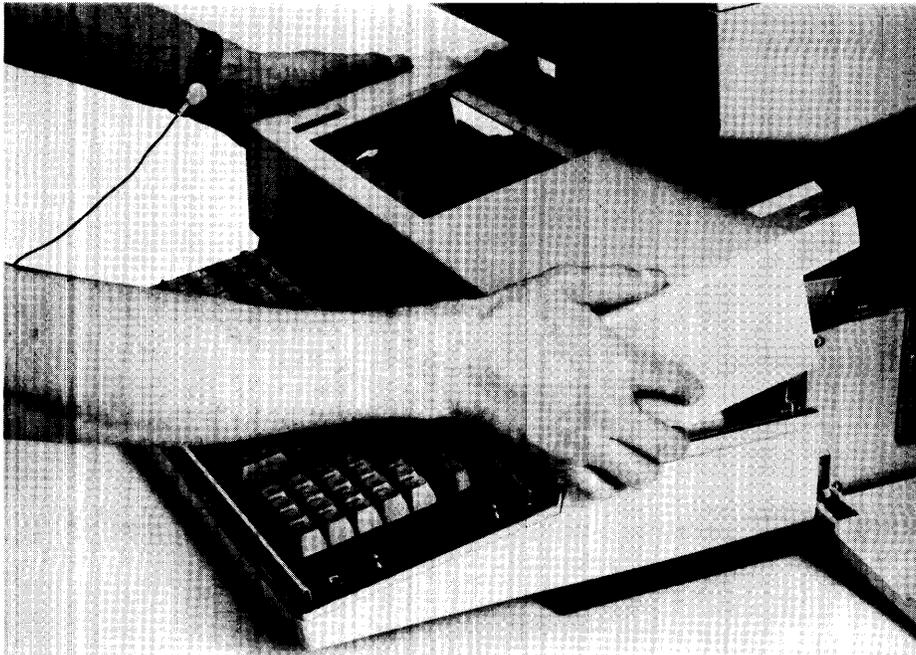
**Figure 4-6. Removing Front Cover**
