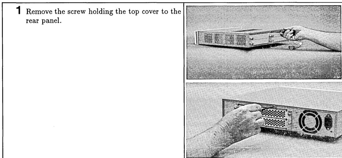
**2** Slide the top cover off to the rear of the expander
