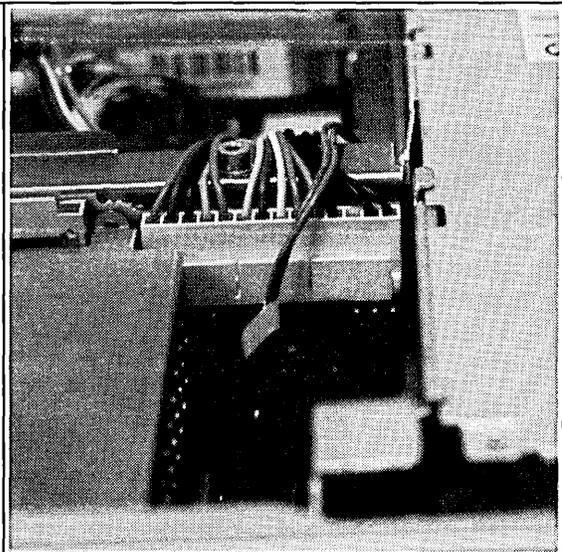
**2** Slide the fan towards the left side and to the front, then lift it out while pulling its wires through the fan wire hole in the power supply.
