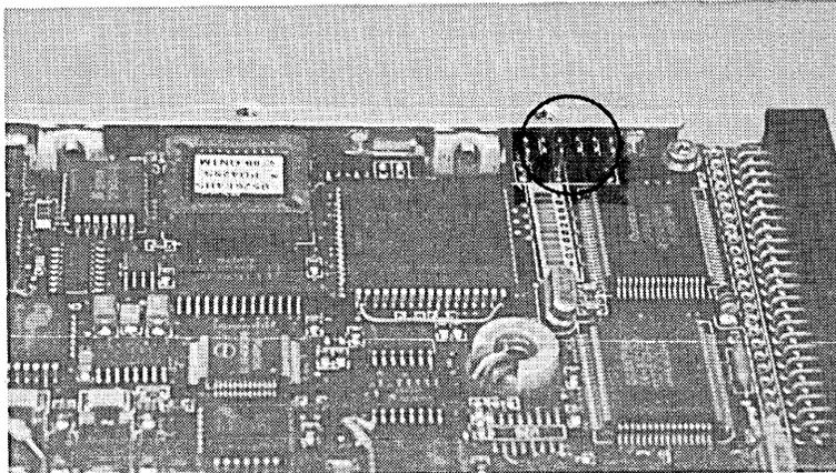
**Figure 5-3. Hard Disk Drive Configuration Jumper Locations**
