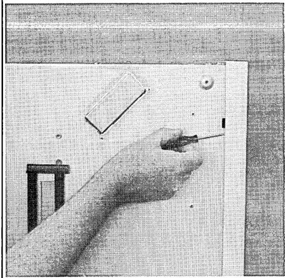
**3** Pull the front panel off the chassis.
