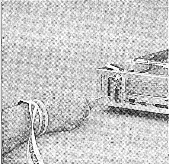
**4** Remove the connector from the rear panel from the inside.
