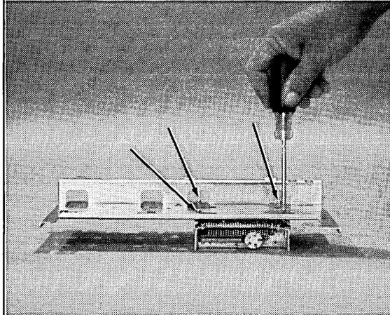
**5** Note the configuration jumper/switch positions. The replacement drive must be configured the same.
