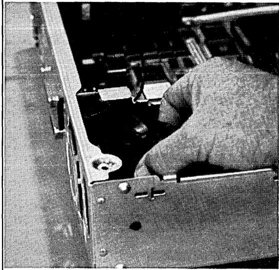
**3** Note the airflow arrow on the fan. When installing the fan, the airflow must be towards the outside.
