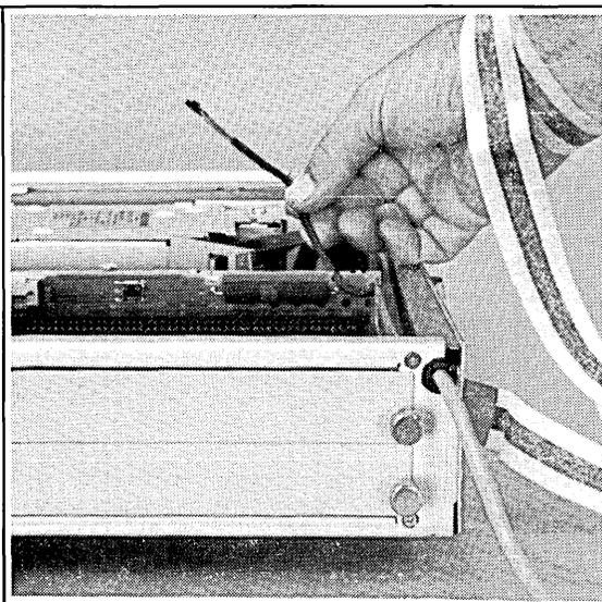
**2** Remove the screw from the fan's cover plate, then lift off the plate.
