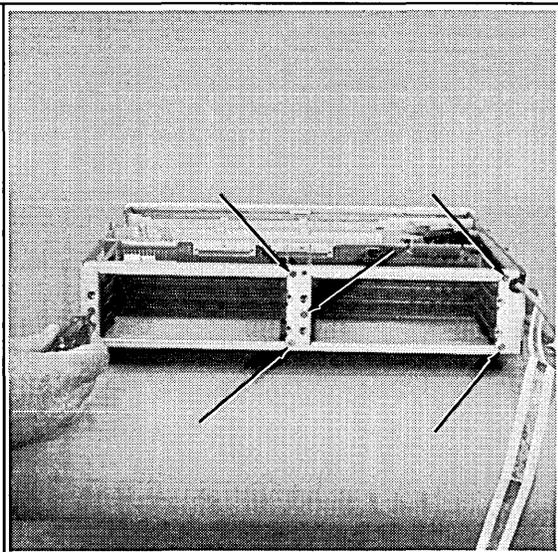
**2** Remove the two screws that go through to the chassis floor.
