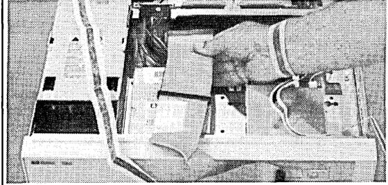
**3** Remove the rear panel's SCSI connector's top and bottom screw.
