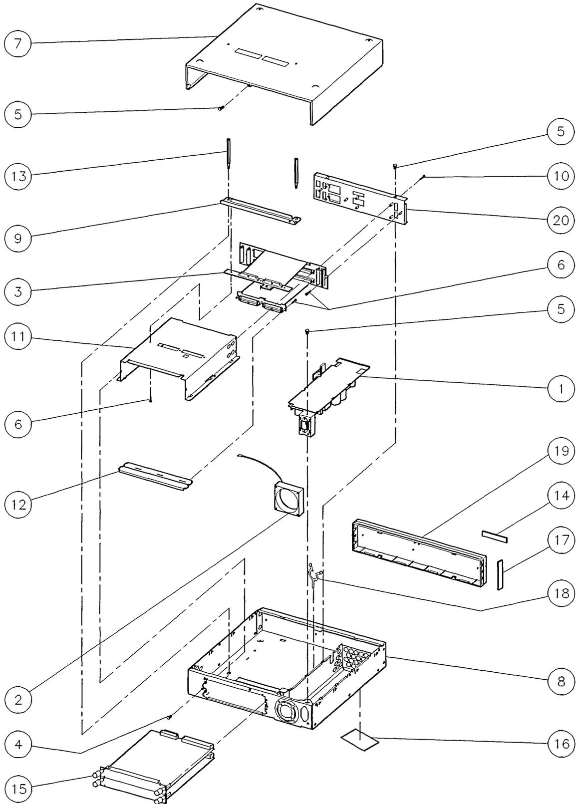
Figure 7-3. HP A2247A DIO-II Bus Expander Exploded View
