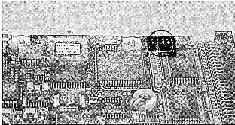
**Figure 5-4. 52 Megabyte Hard Disk Drive Configuration Jumper Locations**
