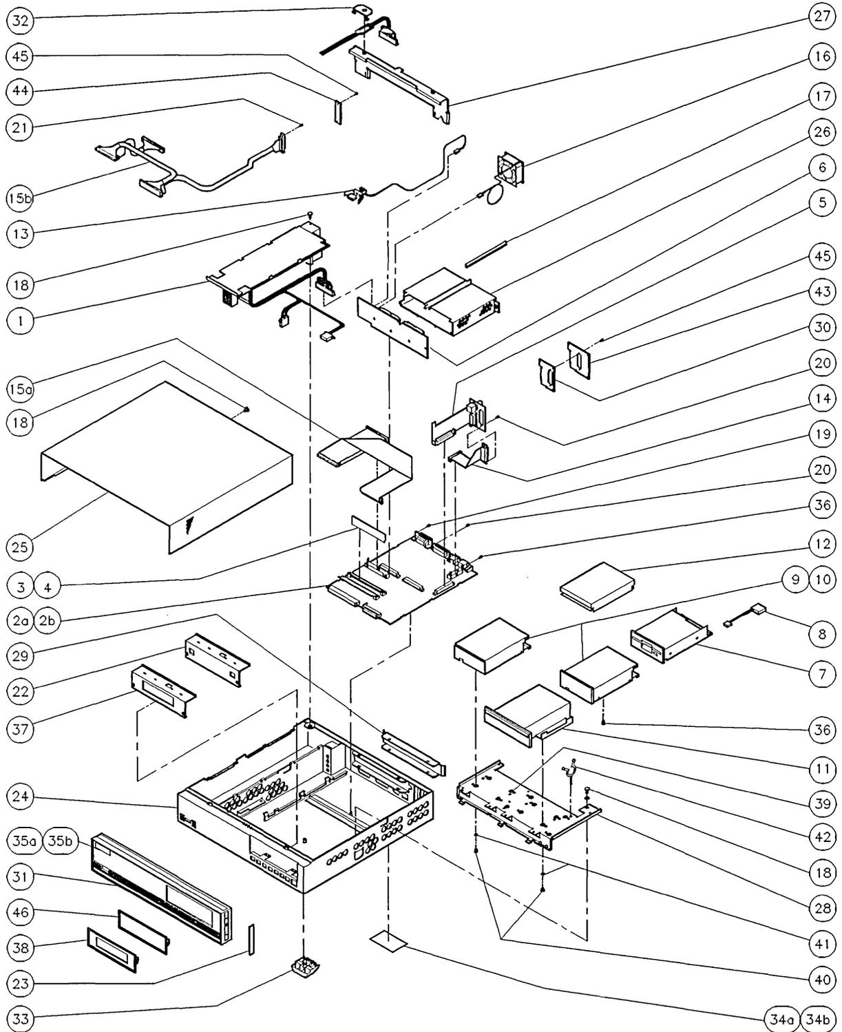
Figure 7-1. Model 362 and 382 Controller Exploded View
