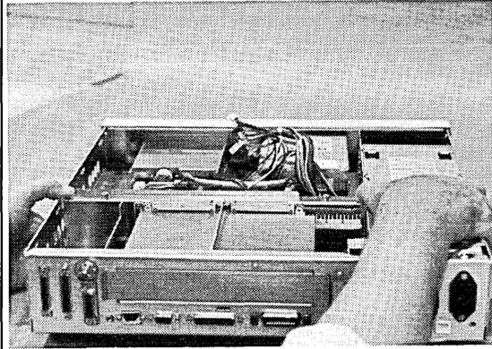
**3** Tilt the support forward about 45° and sliding rearward to unlatch the two hooks at the bottom of the chassis to lift it out.
