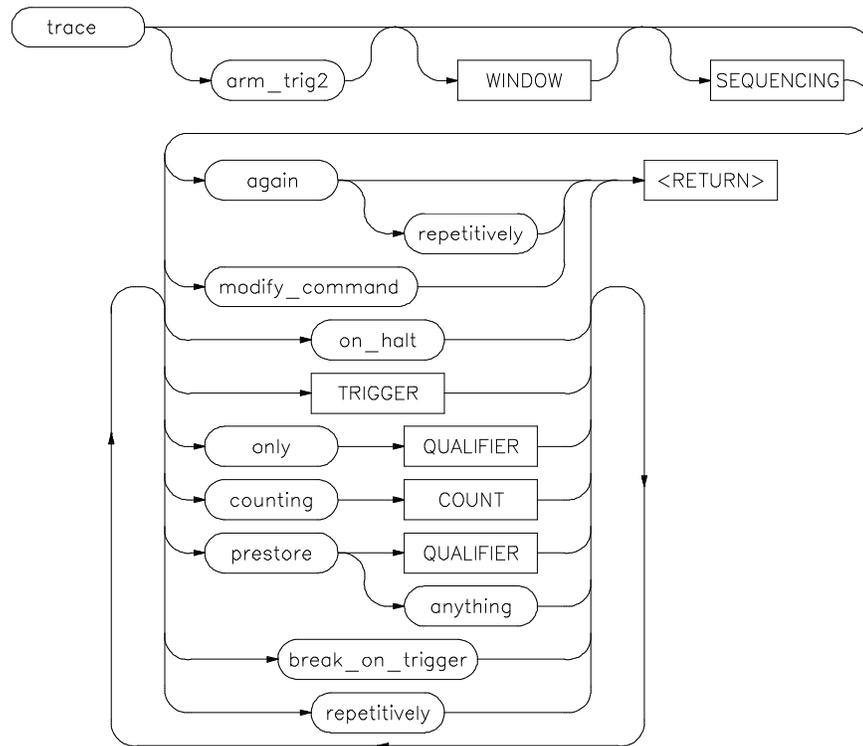
The options shown can be executed once for each **trace** command. Refer to the COUNT, QUALIFIER, SEQUENCING, TRIGGER, and WINDOW diagrams for details on setting up a trace.
