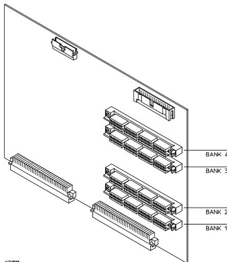
**2** To ensure correct installation of optional memory modules on the deep analyzer card, there is a cutout at one end of the memory modules so they can only be installed the correct way.
