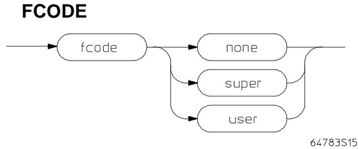
The function code is used to define the address space being referenced. Select the appropriate function code from those listed below.
