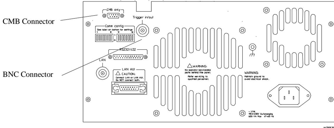
There are three bidirectional signal lines on the CMB connector on the rear panel of the emulator. These CMB signals are:
