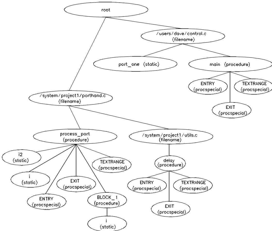
Note that SRU does not build tree nodes for variables that are dynamically allocated on the stack at run-time, such as *i* and *j* within the `delay ()` procedure. SRU has no way of knowing where these variables will be at run time and therefore cannot build a corresponding symbol tree entry with run time address.
