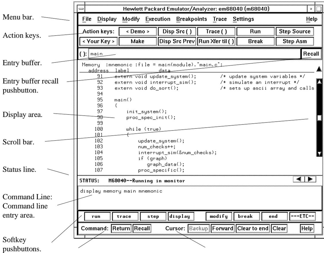
Command pushbuttons. Includes command recall pushbutton.
