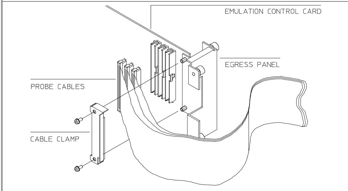
**2** When inserting cable connectors into the sockets, press inward on the connector clips so that they hook into the sockets as shown. The order of connecting cables was given in step 1.
