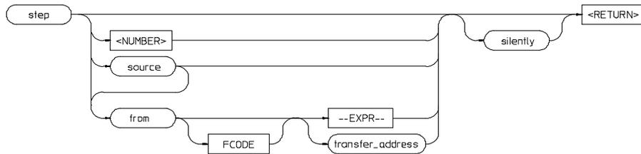
The **step** command allows sequential analysis of program instructions by causing the emulation processor to execute a specified number of assembly instructions or source lines.
