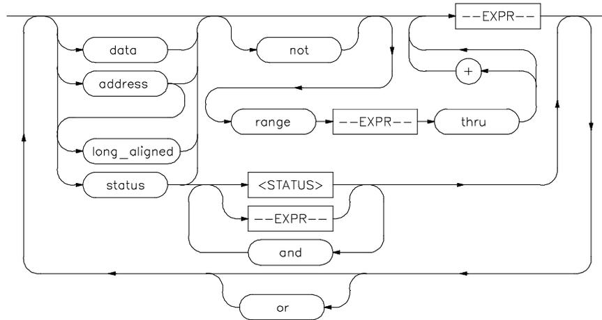
The **QUALIFIER** parameter is used with **trace only**, **trace prestore**, **TRIGGER**, and **trace counting** to specify states captured during the trace measurement.
