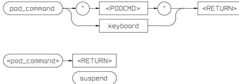
The HP 64700 Series emulators contain a low-level Terminal Interface, which allows you to control the emulator's functions directly. You can issue Terminal Interface commands through the Softkey Interface by using **pod\_command**. With **pod\_command**, you can issue a single command, or enter the keyboard mode which allows you to enter a series of commands.
