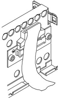
**9** To remove the analyzer card, insert a flat blade screwdriver in the access hole and eject the analyzer card by rotating the screwdriver.
