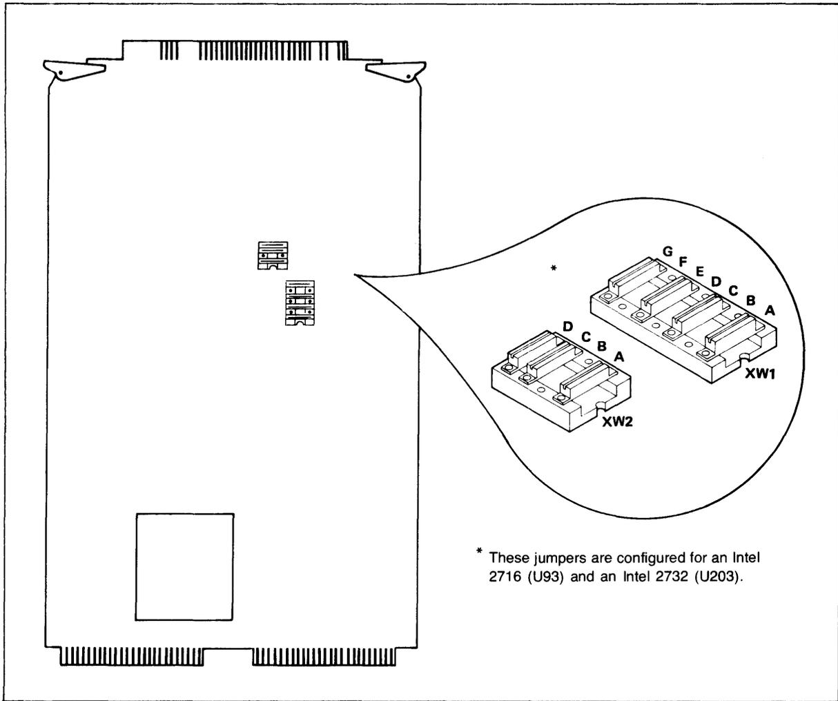
Fig. 2-2. ROM Configuration Jumper Positions
