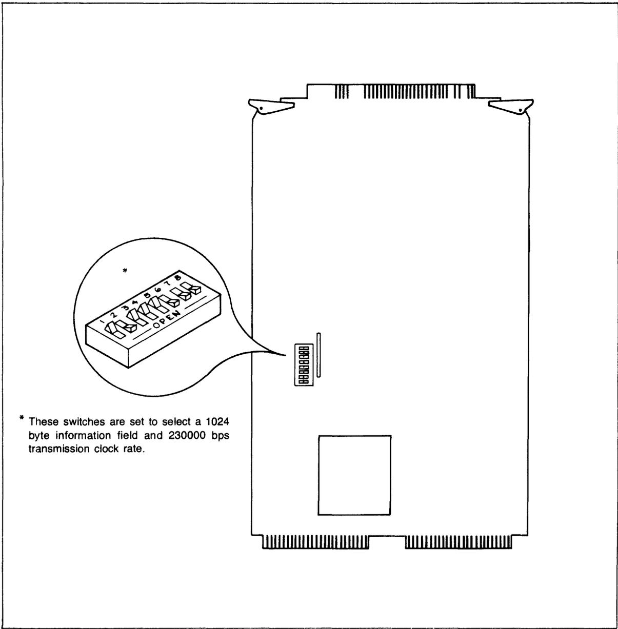
Figure 2-3. DIP Switch Position and Configuration
