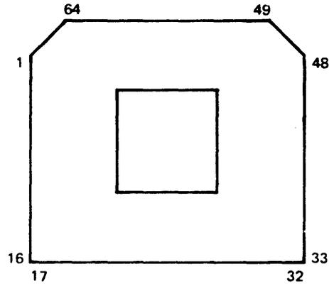
1AC5-6001 I/O PROCESSOR (IOP) CHIP OUTLINE (COMPONENT SIDE)
