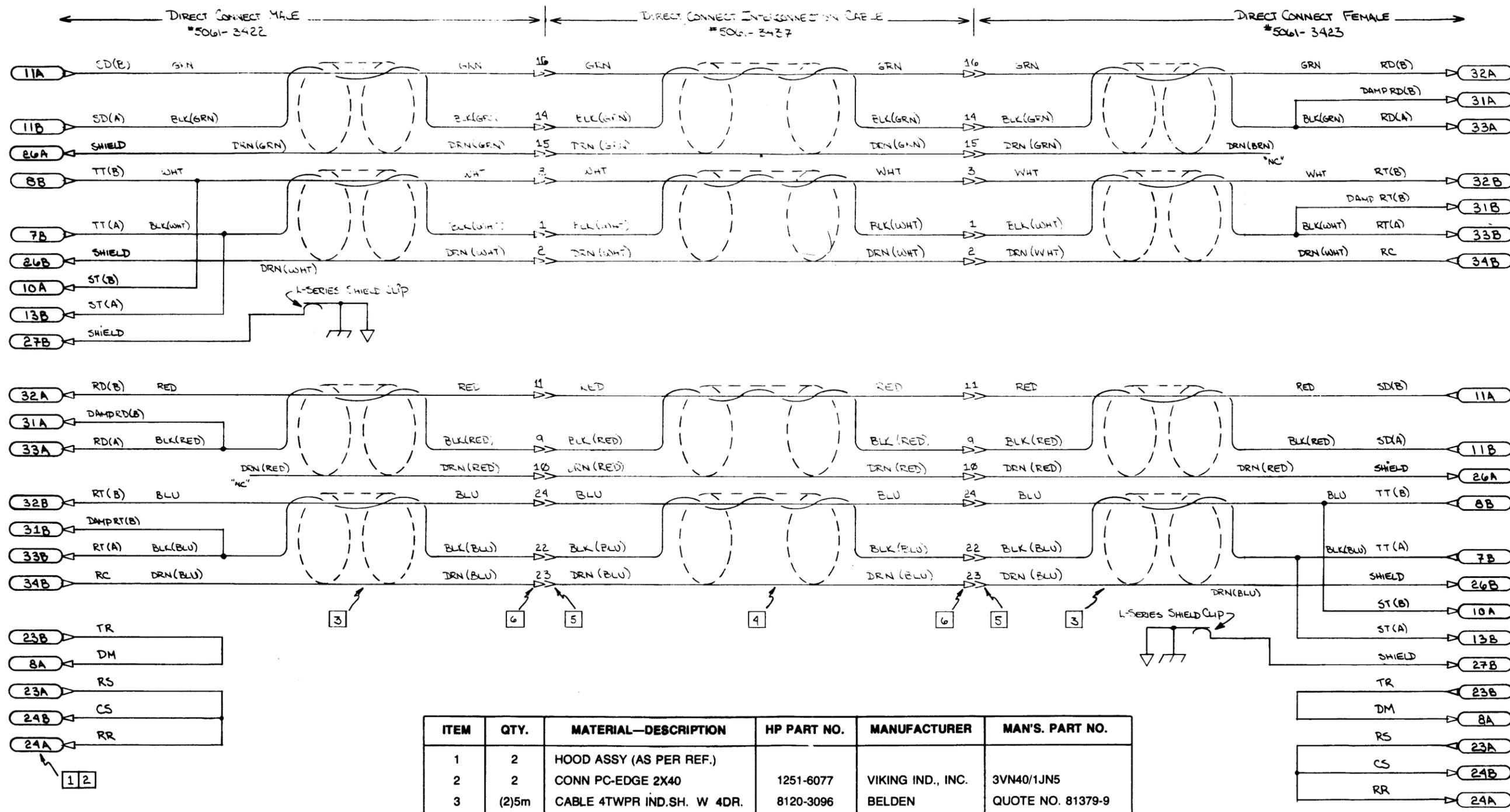
Figure 7-2. Direct-Connect Cable Wiring Diagram.
