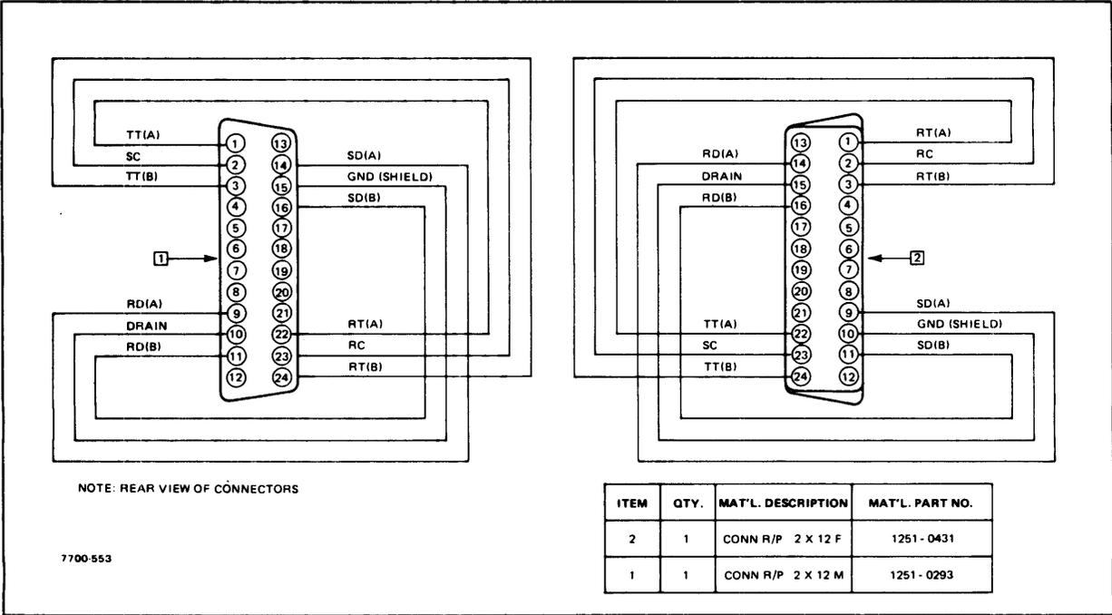
Figure 7-3. Loop-Back Test Connector Wiring Diagram.
