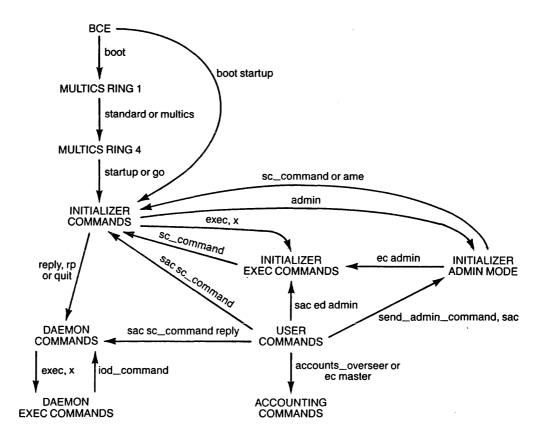
Figure 1-1. Moving From One Command Environment to Another
