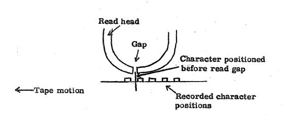
Step 1. Position of tape pre-positioned for reading but before read step.
