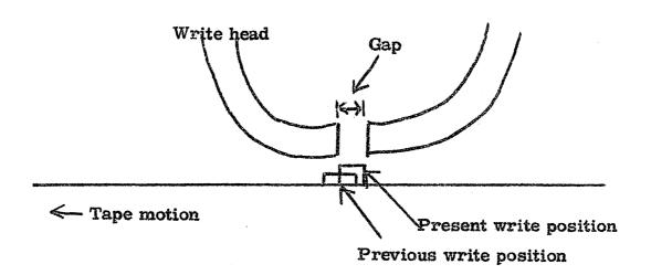
Tape advances . 005" for 200 bpi recording density Tape advances . 0018" for 556 bpi recording density
