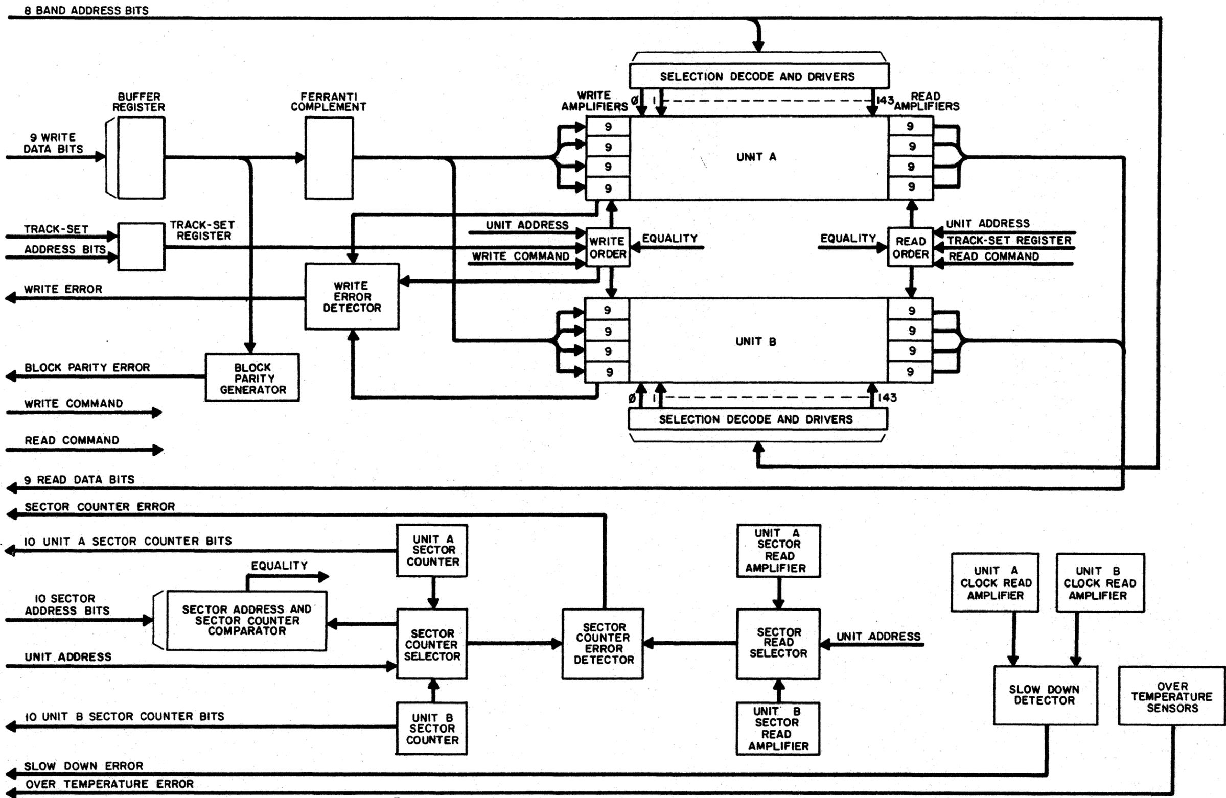
Figure 2-1. LRL Disc System Block Diagram
