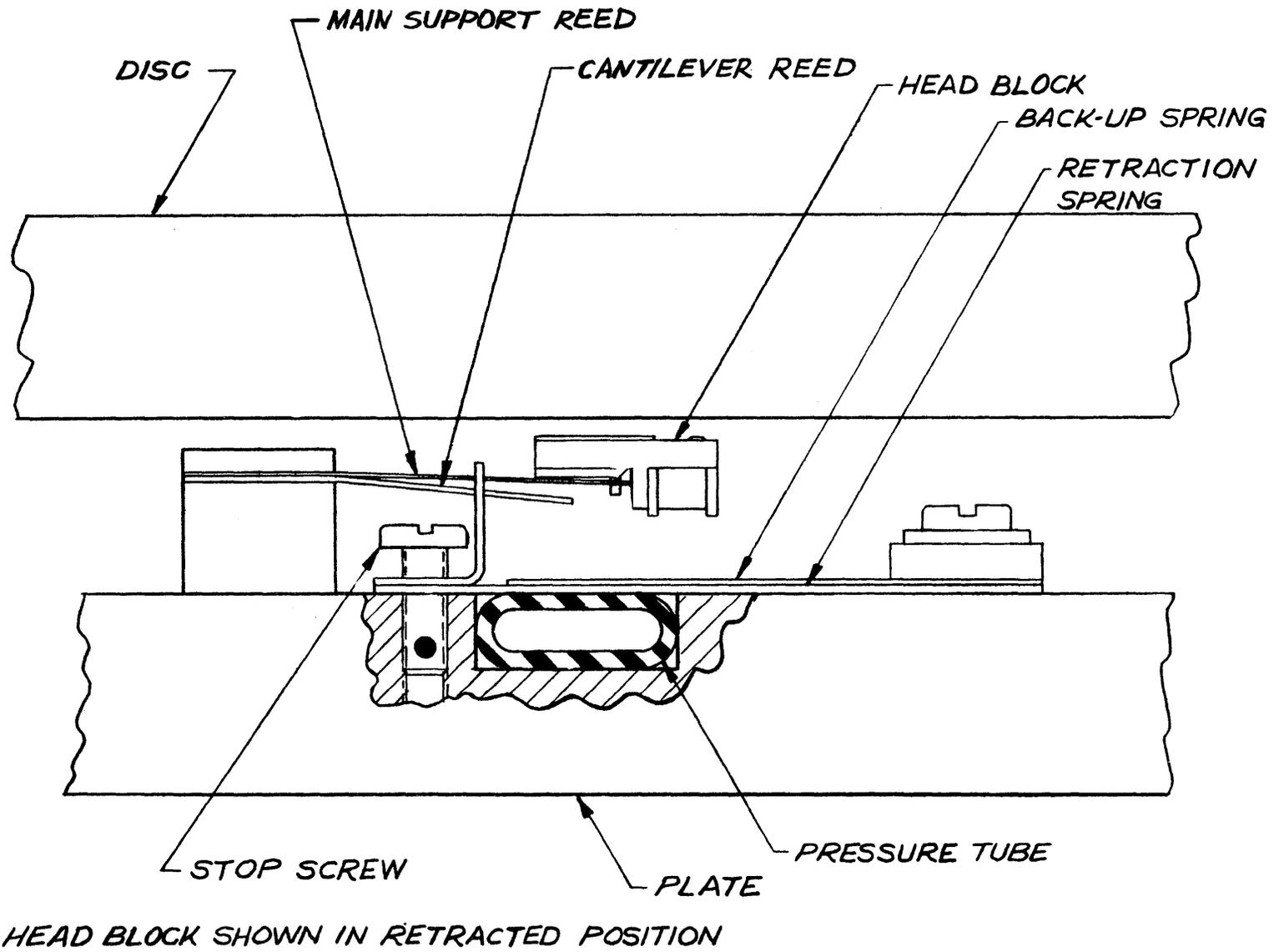
Figure 2-12. AN/FYQ-11 Head Retraction Mechanism
