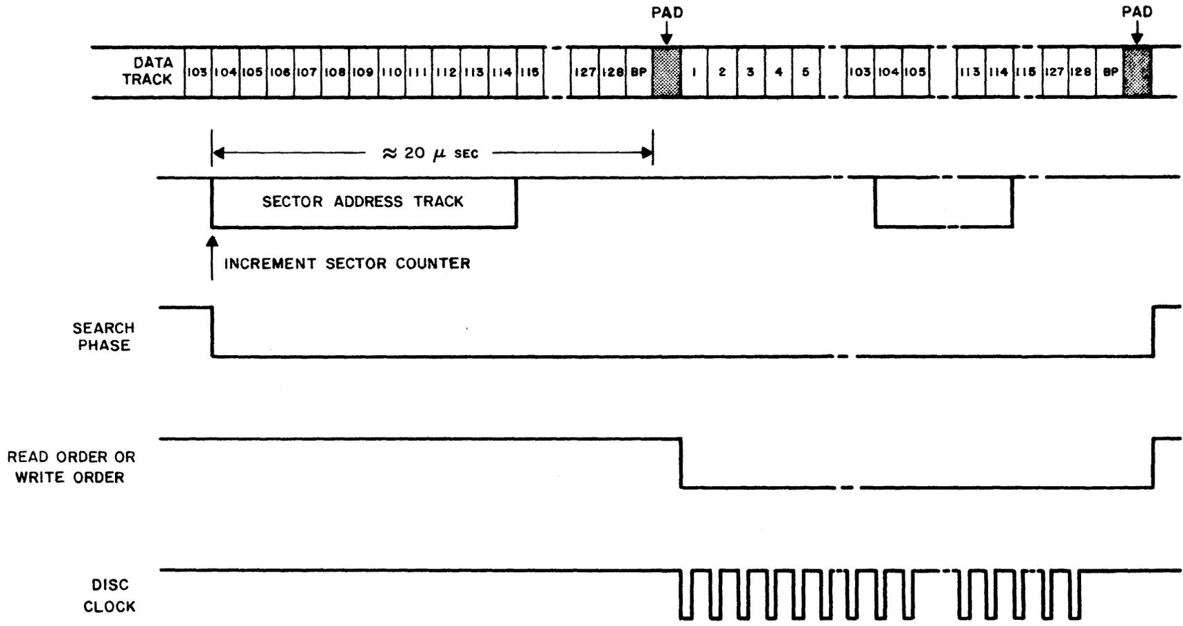
Figure 2-2. Disc Timing Diagram
