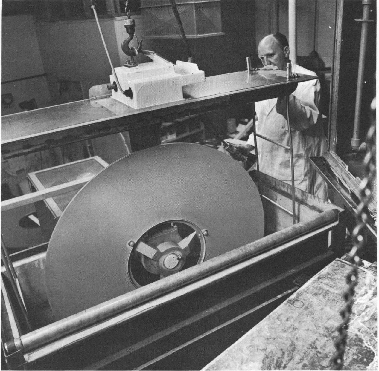
Disc is Lowered into Plating Tank for Application
