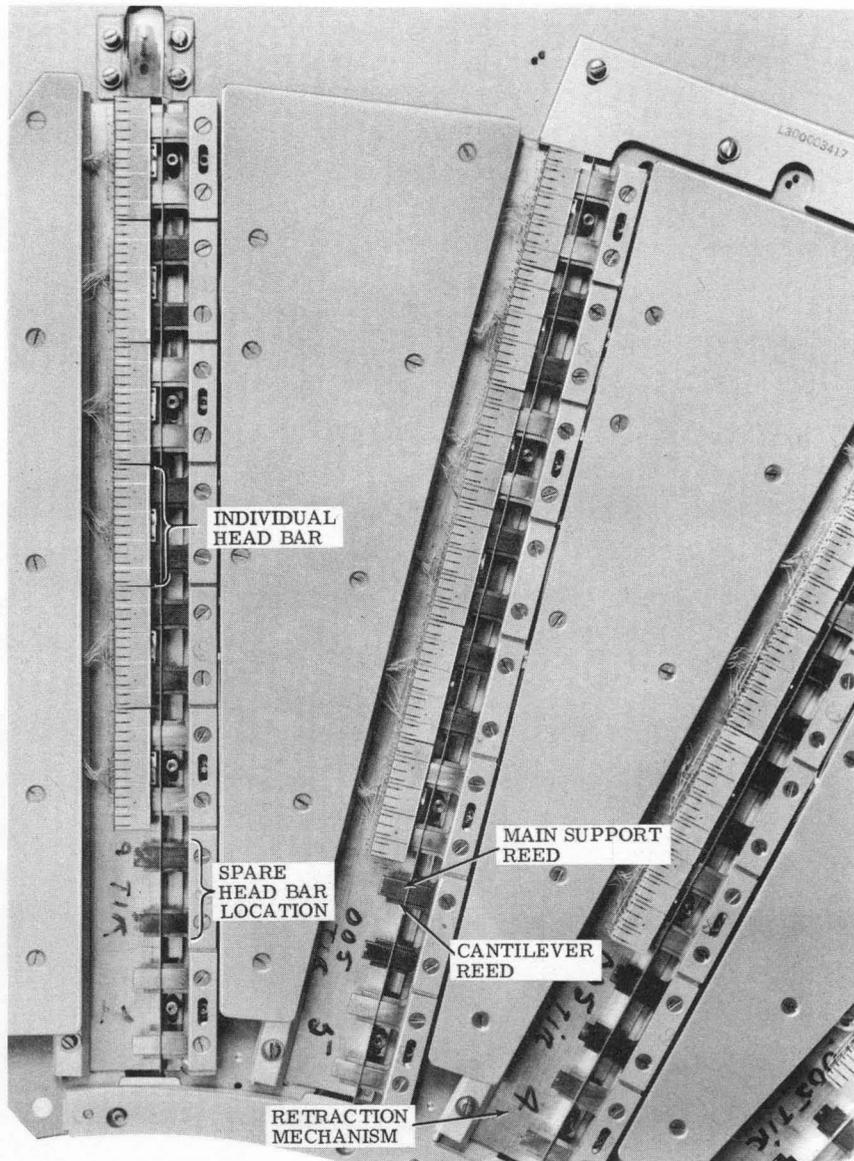
Detailed Section of Head Mounting Plate
