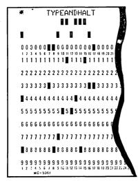
Use: This card causes the contents of the next card to be typed on the console typewriter, and waits in a loop for console switch 19 to be toggled. When switch 19 is toggled, the following card is read.
