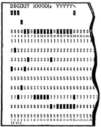
Use: Causes a dump on the high-speed printer of the portion of GE-225 memory specified by beginning octal address xxxxx and ending octal address yyyyy.
