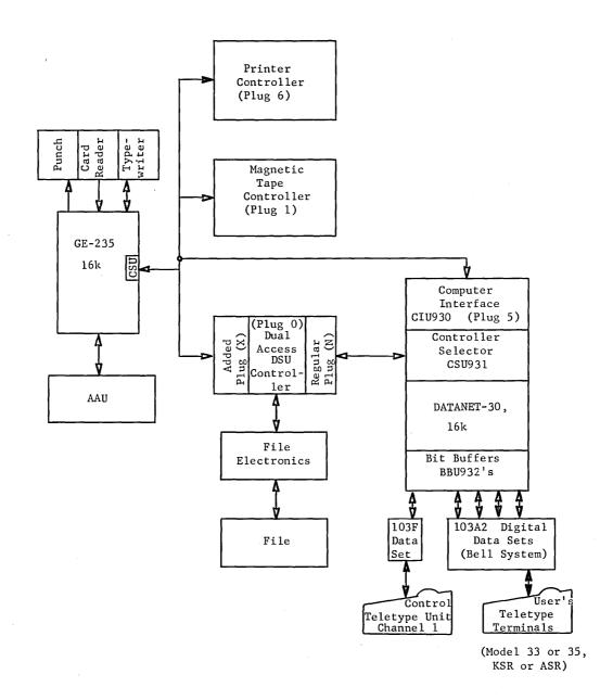
Figure 2. GE-265 Time-Sharing System Cabling
