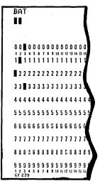
Use: Causes the decimal card deck in the card reader to be written as 27-word card images in the binary mode onto tape 4. Card-to-tape operation terminates on detection of a "quote" card or a hopper empty condition. "Quote" cards have 0-7-8 punches in columns 1-6. Upon termination, the program writes an end-of-file mark on tape 4 and rewinds it.
