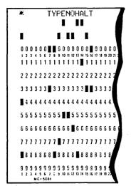
Use: This card causes the contents of the next card to be typed on the console typewriter, then reads the following card.
