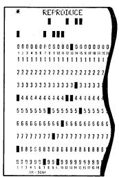
Use: This card causes the deck in the card reader to be reproduced in the card punch. Reproduction is terminated on a hopper empty condition. The deck to be reproduced should be followed by two blank cards.
