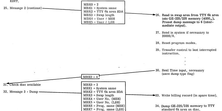
Figure 9. Internal Processing of RUN
