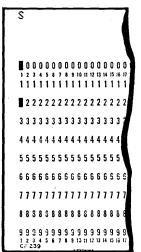
Use: Halts the GE-225 and makes the card reader available for program input. The S-card must precede other commands. Toggle Switch 18 to initiate reading of the S-card. (Also stops the currently running background program in the GE-225.)
