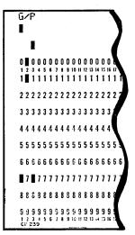
e: Results in the exact reproduction of a deck from the card reader to the card punch. Punching terminates on a hopper-empty condition.
