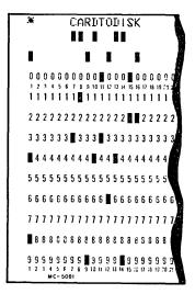
Use: This card causes the Exec to call the card to disc (CTD) program from the disc and turn control over to it. CTD then loads the background program immediately following the \* CARDTO-DISK card in the card reader onto the disc, making the proper entries into the background card catalog. This enables the user to store frequently used background programs on the disc, instead of loading them with a \* BINARY control card each time they are run.
