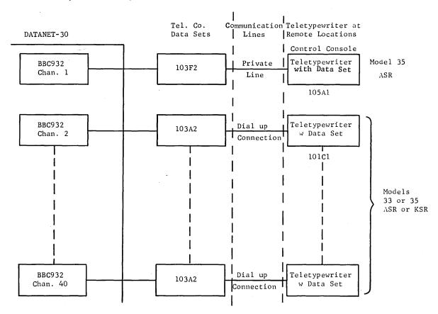
Figure 13. Interface Communications Hardware
