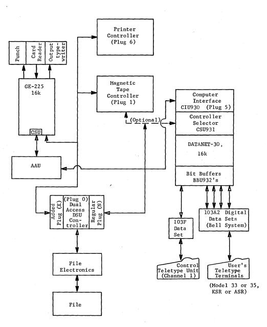
Figure 1. GE-255 Time-Sharing System Cabling
