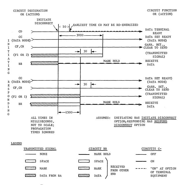
Figure 17. Data Set 103A Space Disconnect Sequence
