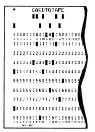
Use: This card causes the decimal card deck in the reader to be written as 27-word card images onto tape 4, in the binary mode. Card-to-tape operation will terminate on finding a "quote" card, or on a hopper empty condition. "Quote" cards have 0-7-8 punches in columns 1-6. On terminating, the program writes an end-of-file on tape 4 and rewinds it. \* TYPEANDHALT
