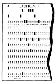
Use: This card causes the deck in the card reader to be listed on the on-line printer with parentheses and other special characters converted for printer compatibility. Listing will be terminated on a hopper empty condition. The deck must be followed by two blank cards.
