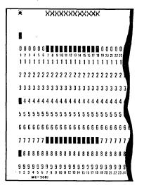
Use: This card causes the Exec to search the background card catalog for a background program whose name as given in its header is xxxxxxxxx. When this entry is found, the Disc Card Image Loader (DCIL) program is read in as an overlay to the Exec. The DCIL then loads the background program from the disc into memory, and turns control over to it.
