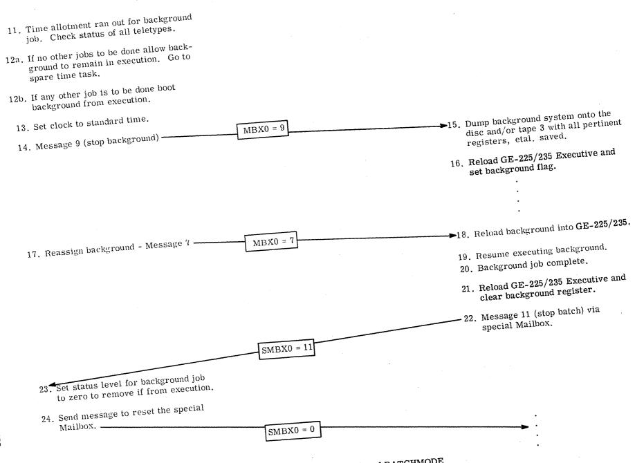
Figure 10. Internal Processing of BATCHMODE
