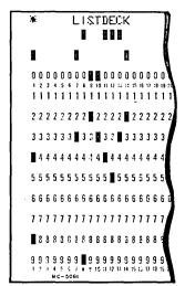
Use: This card causes the deck in the card reader to be listed on the on-line printer. Listing is terminated by a hopper empty condition. Parentheses and other special characters will not be translated for printer compatibility. The deck must be followed by two blank cards.
