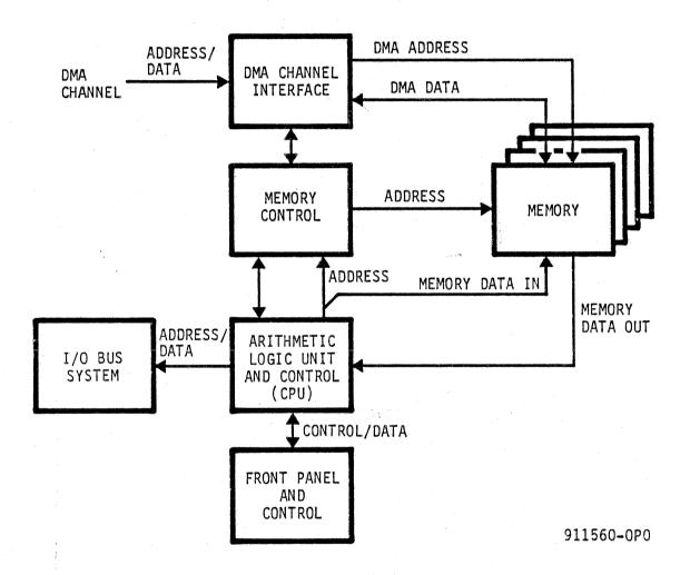
FIGURE 2-1 SPC9800 COMPUTER BLOCK DIAGRAM
