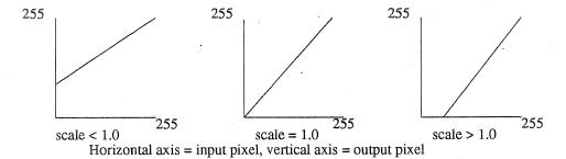
As the diagram indicates when **scale** is less than 1.0 (between 0.0 and 1.0) the output pixel values start out greater than 0 and slowly go to maximum. When **scale** is equal to 1.0 it is a direct map of input values to output values. And finally when **scale** is greater than 1.0 the smaller input values map to a 0 output value (to a certain point) then output values increase rapidly to maximum.
