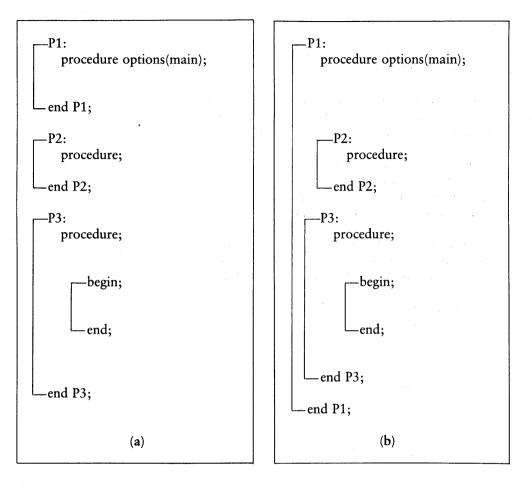
Figure 2-2. Internal and External Blocks
