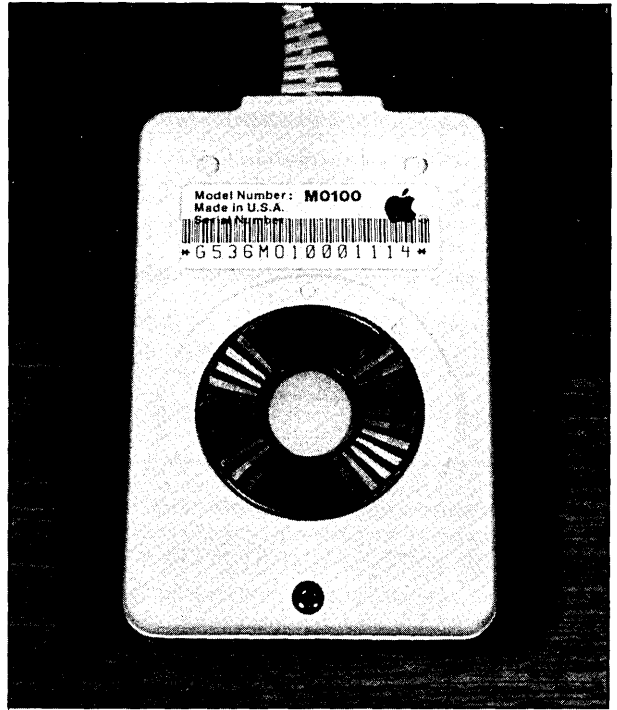
Fig. 2-2. A typical mechanical mouse. A rolling ball is used for control in this mouse. The Macintosh mouse is a good example of a mechanical mouse.
