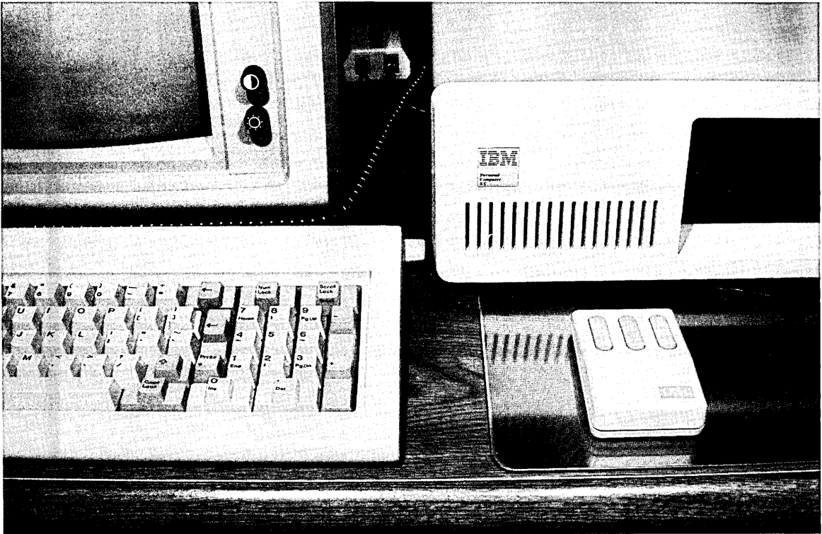
Fig. 2-1. A complete GEM system: the IBM PC XT, Hercules Graphics Card, IBM Monochrome Display, and Mouse Systems mouse.
