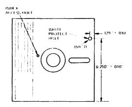
Figure 33. Write Protect Hole Specifications
