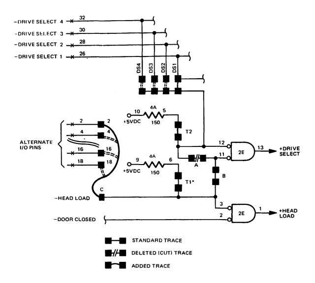
IF THE —HEAD LOAD LINE IS MULTIPLEXED, TERMINATOR 'T1' MUST BE CUT ON EACH DRIVE EXCEPT THE LAST ONE ON THE LINE.
