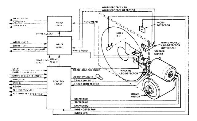
Figure 2. SA800/801 Functional Diagram
