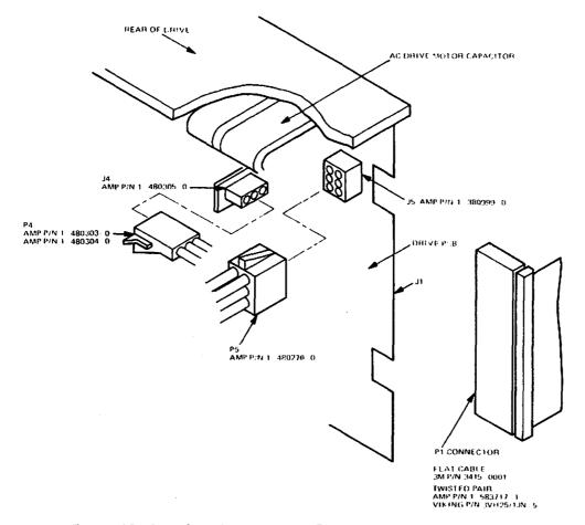
Figure 16. Interface Connectors — Physical Location Diagram
