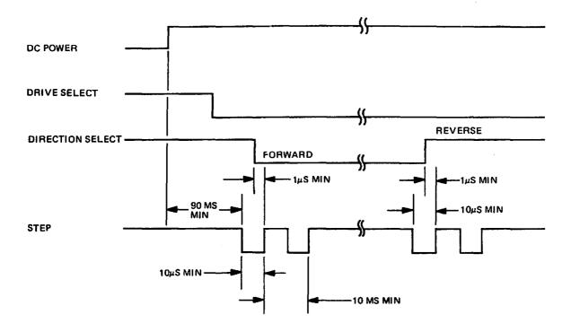
Figure 3. Track Access Timing
