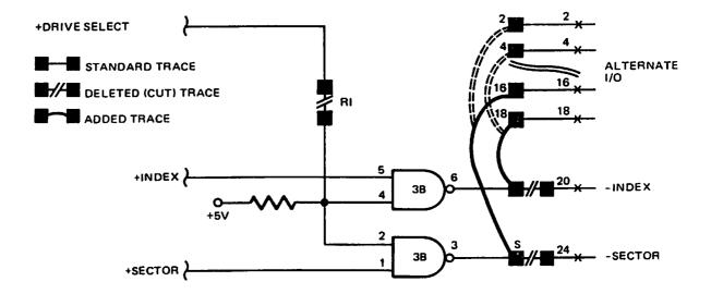
Figure 26. Radial Index/Sector Circuit
