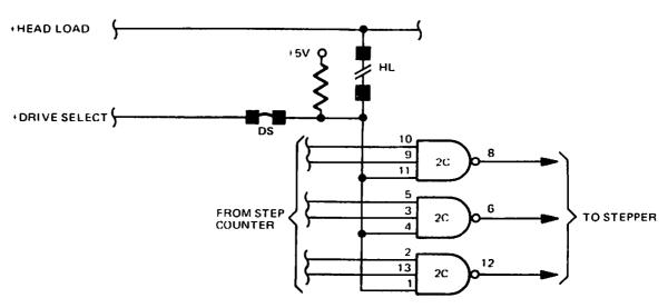
Figure 23. Stepper Motor Enable Circuit
