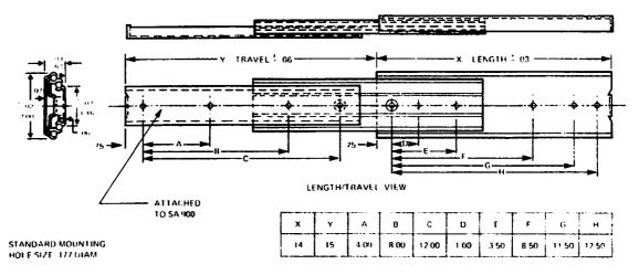
Figure 19. Slide Mounting Dimensions
