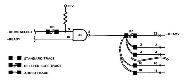
Figure 25. Radial Ready Circuit
