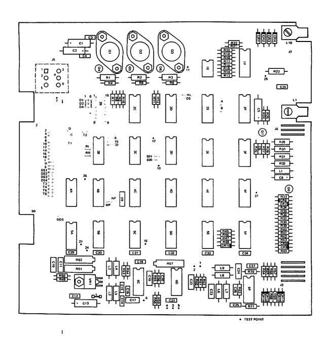
Figure 20. SA800/801 PCB Component Locations
