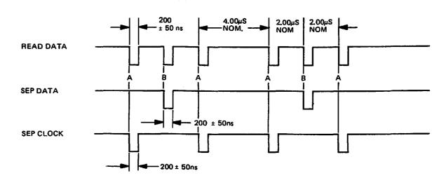
A = LEADING EDGE OF BIT MAYBE ± 400 ns FROM ITS NOMINAL POSITION. B = LEADING EDGE OF BIT MAYBE ± 200 ns FROM ITS NOMINAL POSITION.
