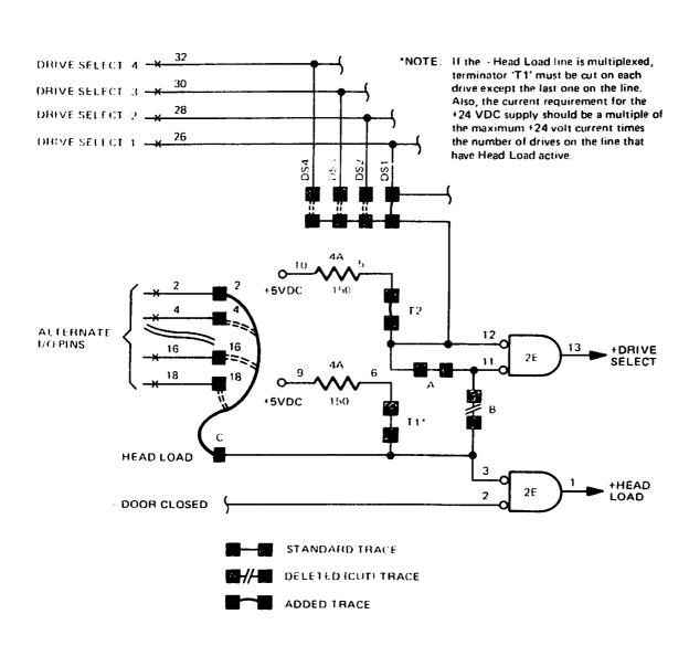
Figure 22. Select Drive Without Loading Head Circuit
