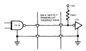
Figure 10. Interface Signal Driver/Receiver
