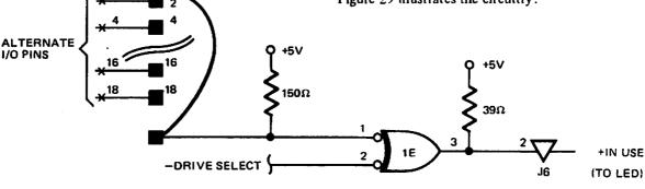
Figure 29. In Use/Activity LED Circuit
