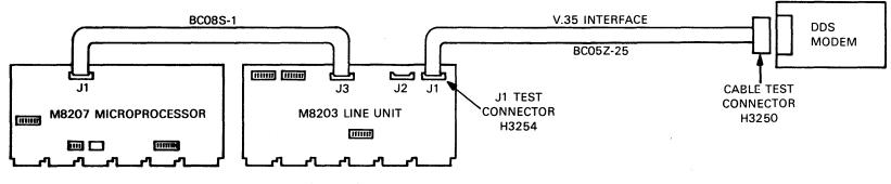
Figure 2-8 DMP11 Remote System Cabling Diagram (Sheet 2 of 2)
