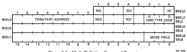
Figure 3-5 Mode Definition Command Format
