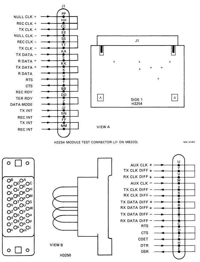
Figure 2-7 DMP11 Turnaround Test Connectors (Sheet 1 of 4)
