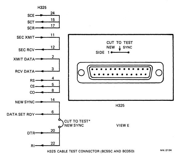
Figure 2-7 DMP11 Turnaround Test Connectors (Sheet 4 of 4)
