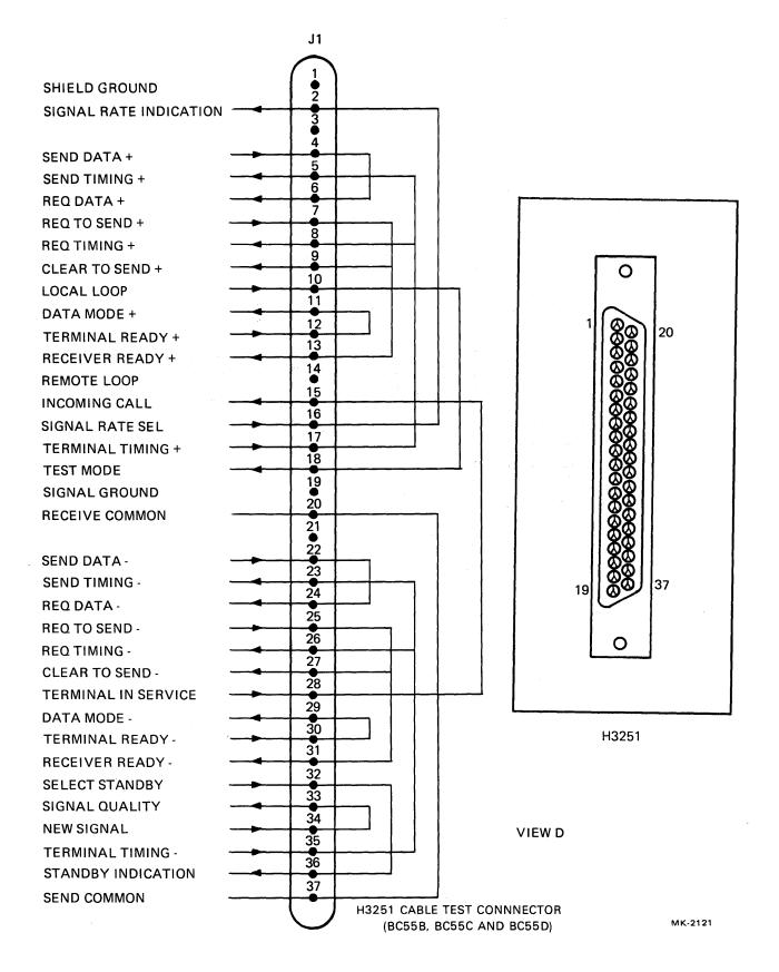
Figure 2-7 DMP11 Turnaround Test Connectors (Sheet 3 of 4)
