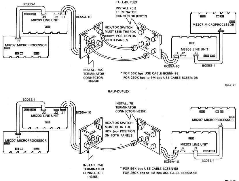
Figure 2-10 Multipoint Cable Routing Example Half-Duplex
