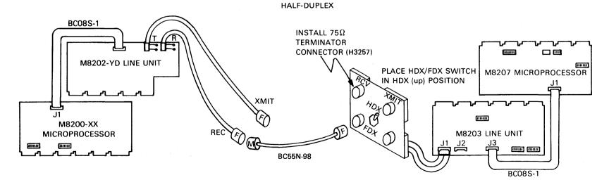
Figure 2-9 DMC11 to DMP11 Integral (Local) Modem Cabling Diagram for Point-to-Point Network
