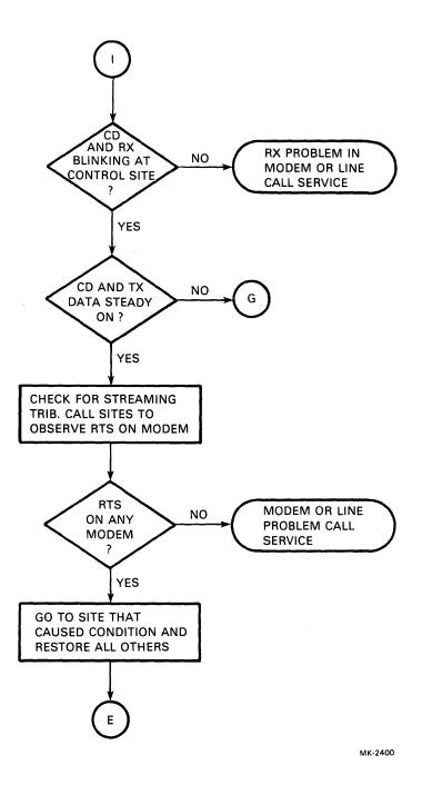
Figure 6-1 Typical Isolation Troubleshooting Flowchart (Sheet 3 of 5)
