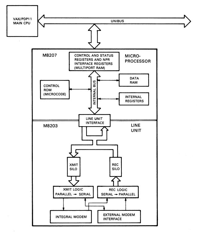
Figure 1-1 Simplified Block Diagram
