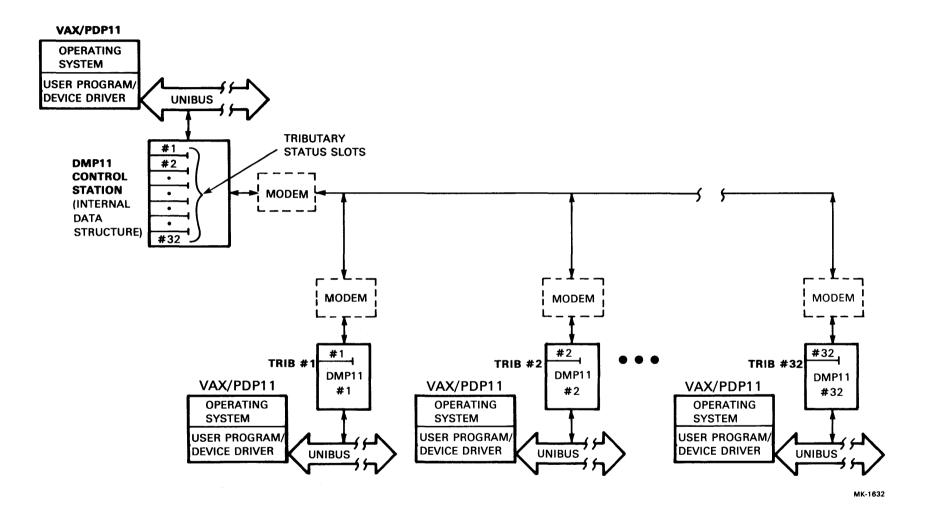
Figure 1-3 Block Diagram of a Multipoint Network with Single Assigned Addresses
