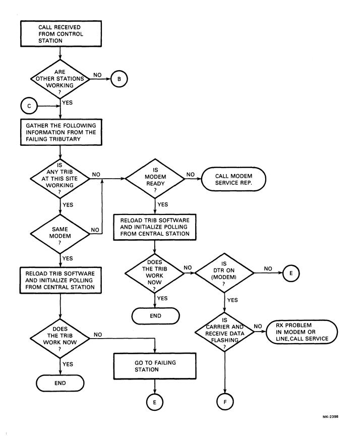
Figure 6-1 Typical Isolation Troubleshooting Flowchart (Sheet 1 of 5)
