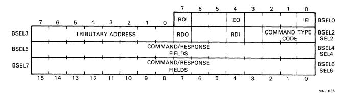
Figure 3-2 Command and Response Fixed and Variable Formats
