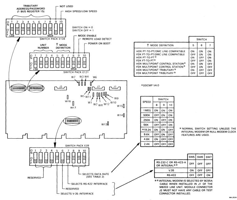
Figure 2-4 M8203 Switch and Jumper Locations
