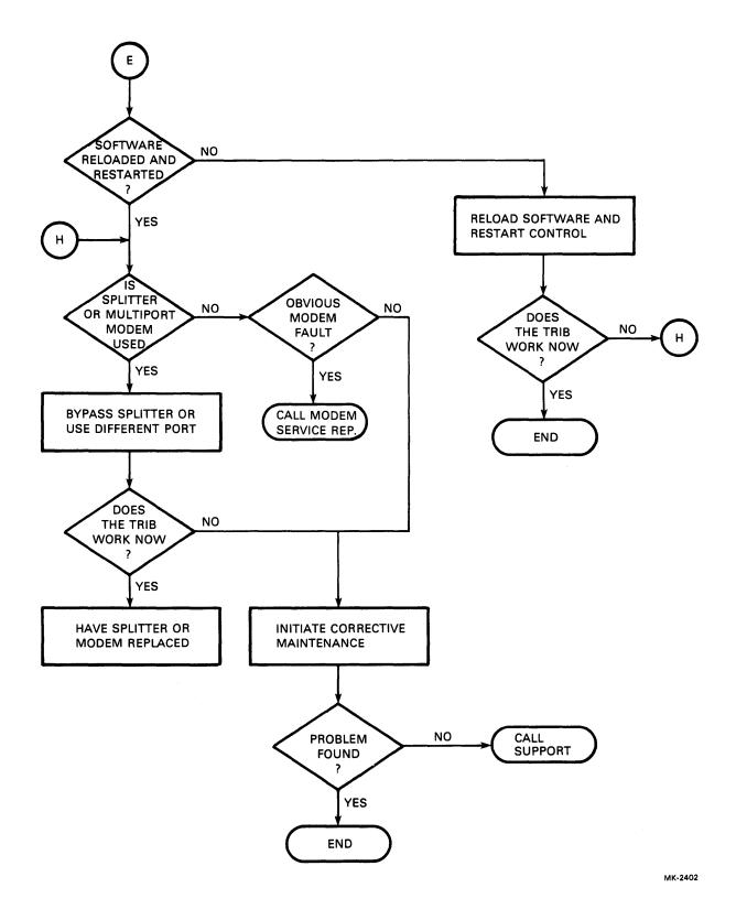
Figure 6-1 Typical Isolation Troubleshooting Flowchart (Sheet 5 of 5)
