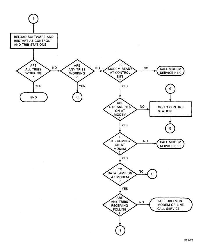
Figure 6-1 Typical Isolation Troubleshooting Flowchart (Sheet 2 of 5)
