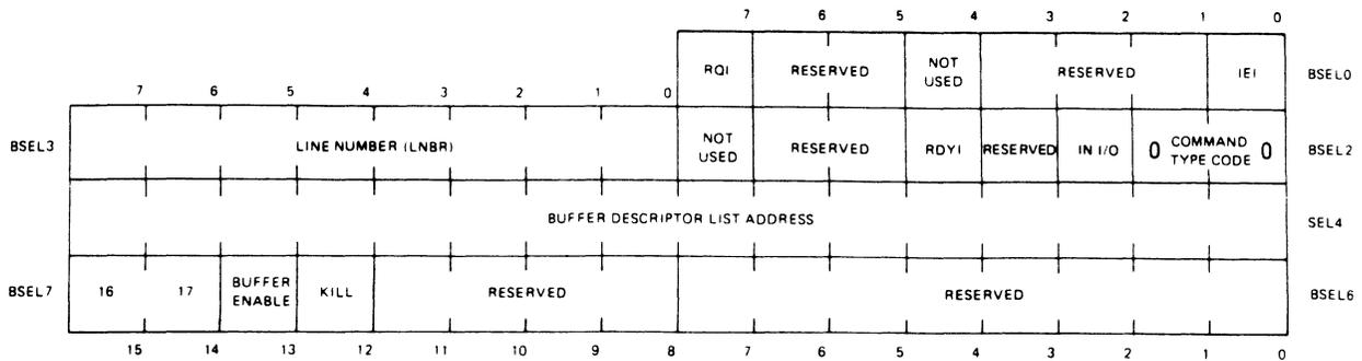
Figure 2-5 BUFFER ADDRESS IN Command Format
