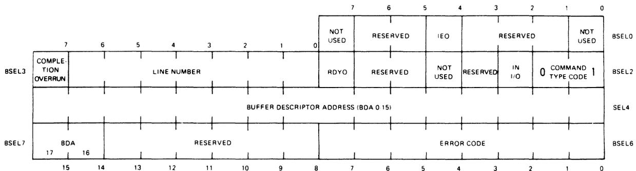
Figure 2-7 CONTROL OUT Command Format
