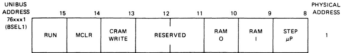
Figure 4-1 Control and Status Register CSr1 Bit Map
