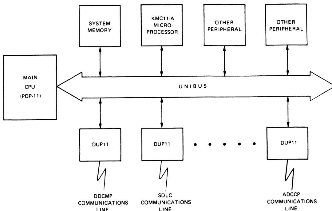
Figure 1-1 COMM IOP-DUP Synchronous Communications Line Controller Configuration
