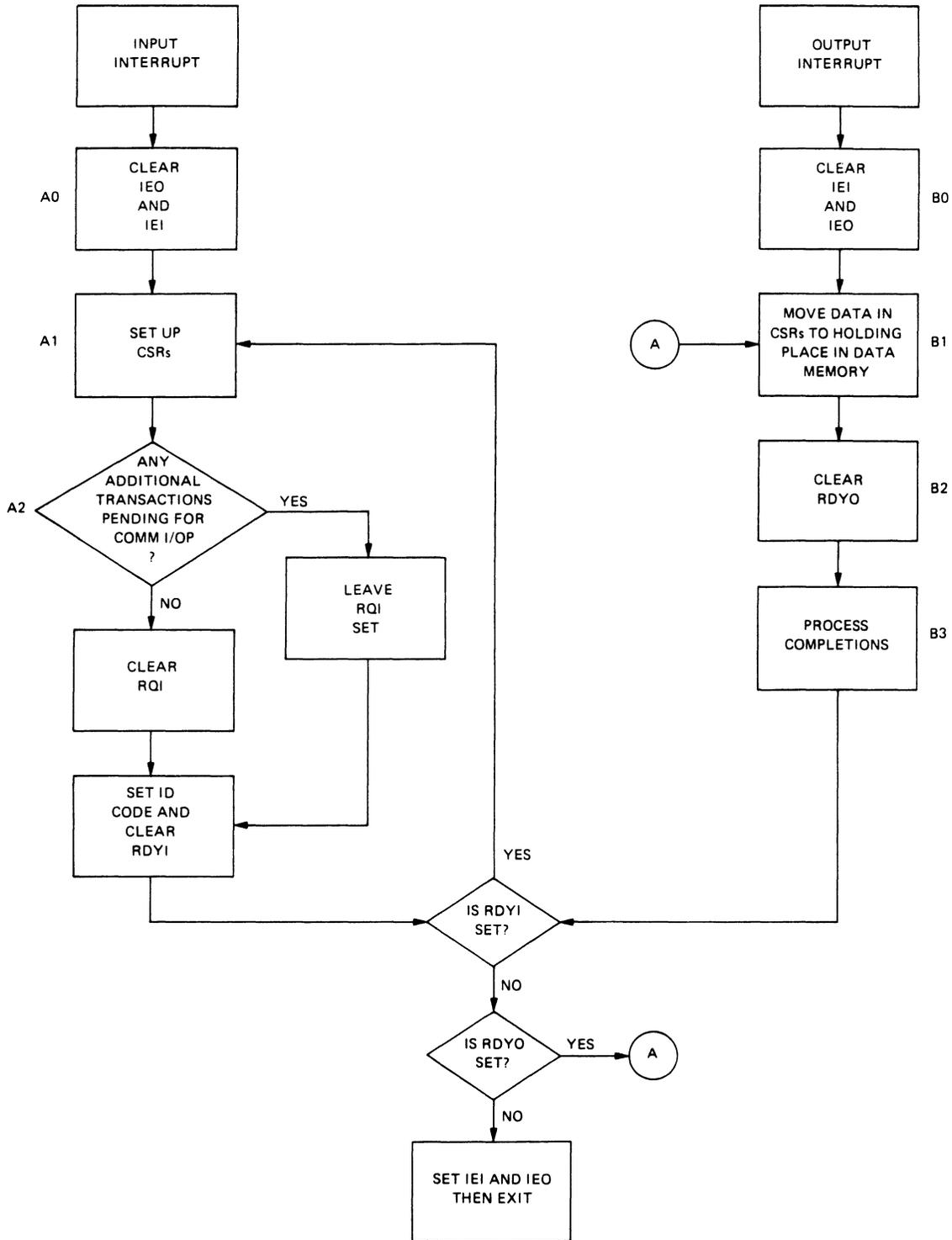
Figure A-1 Flow Chart of a User Program Routine to Handle COMM IOP-DUP Interrupt Processing
