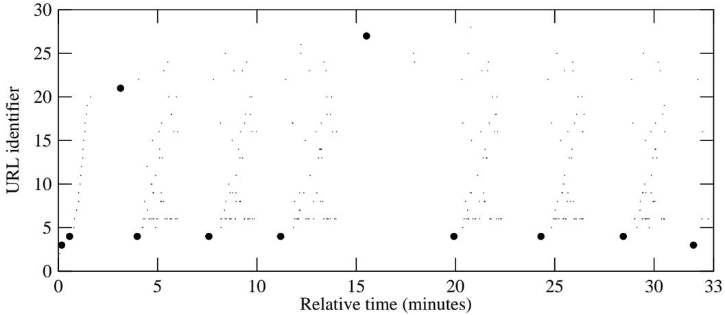
**Figure 5-7:** Timeline showing lack of any client caching
