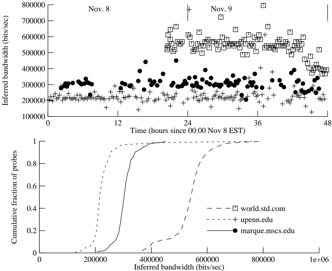
**Figure 6-8:** Network bandwidths inferred from periodic probes
