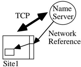
where `"obj"` is the registration name for the object, `site1Obj` is the object, and `NameServer` is a string containing the net IP address or IP name of the machine running the desired name server. (The empty string can be used as an abbreviation for the local IP address.) The object is now available through the name server, as long as the site that exports it is alive. Objects and engines (section 3.8) are the only Obliq values that can be exported to name servers.
