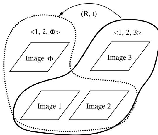
Figure 11: Scheme for generating a novel view (adapted from [2]). Images 1, 2, and 3 are the reference images while image  $\Phi$  is the novel image to be synthesized.  $(R, t)$  is the camera transformation from view 3 to view  $\Phi$ .
