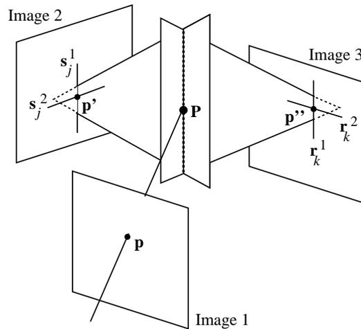
Figure 10: Interpretation of the trilinear tensor (adapted from [2]).  $\mathbf{P}$  is the 3-D point with  $\mathbf{p}$ ,  $\mathbf{p}'$ , and  $\mathbf{p}''$  being the projected image points of  $\mathbf{P}$ .
