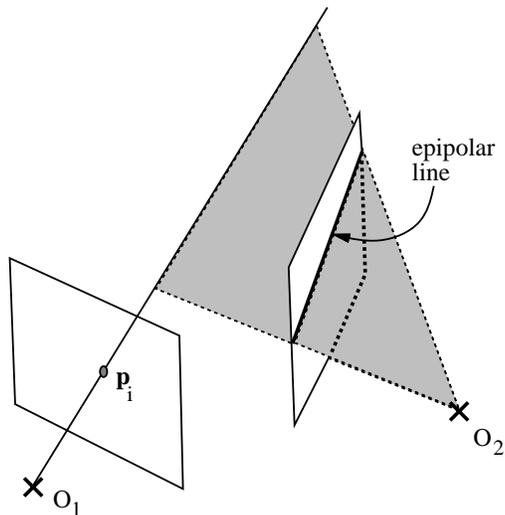
Figure 7: The epipolar constraint on a pair of images. The  $\times$ 's are the camera optical centers. For a given point in one image, the location of the corresponding point in the other image is constrained to lie on a line called the epipolar line.
