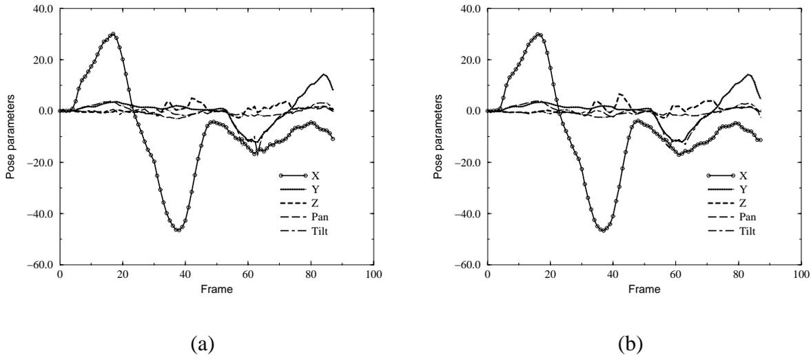
Figure 7: Pose parameter against time for head motion in predominantly X and then Y image plane directions. (a) and (b) are the unfiltered and filtered versions respectively.
