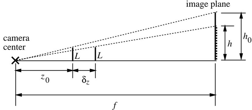
Figure 4: Effect of moving along the camera axis.  $f$  is the camera focal length,  $L$  is the length of the object,  $z_0$  is the reference location,  $\delta_z$  is the change in object location, and  $h_0$  and  $h$  are the projected images lengths (in pixels) of the object at positions  $z_0$  and  $(z_0 + \delta_z)$  respectively.
