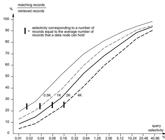
Figure 10:  $hB^{\Pi}$ -tree range search performance in terms of the ratio of retrieved points that satisfy the query over total number of retrieved points per range search, under various node sizes (0.5, 1, 2, and 4 Kbytes) and query selectivity.
