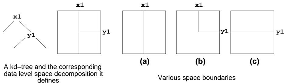
Figure 3: Data level space decomposition and various data and non-data space boundaries.
