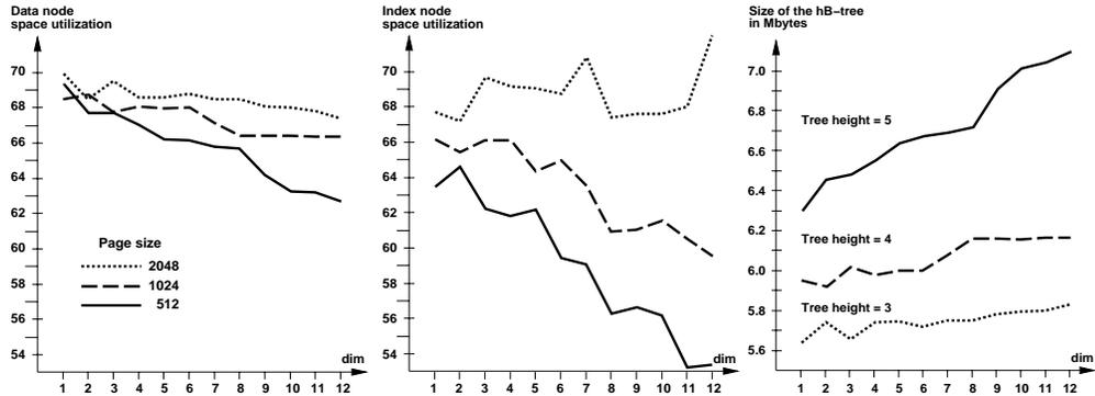
Figure 12: Index and data  $hB^{\Pi}$ -tree node space utilization and size of the  $hB^{\Pi}$ -tree in terms of height and Mbytes under different page sizes and dimensions (indexed attributes). For page sizes greater than 1K bytes the  $hB^{\Pi}$ -tree is fairly insensitive to dimension. (In all cases the same 150,000 24-byte records were inserted with their attribute values following a 90:10 skewed distribution.)
