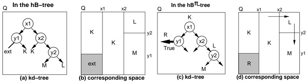
Figure 2: Intra-node organization of hB-tree and hB <sup>$\Pi$</sup> -tree nodes using kd-trees.
