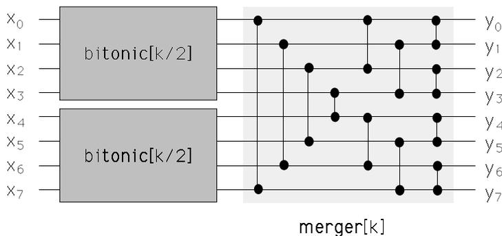
Figure 3: Recursive Structure of a BITONIC[8] Counting Network.
