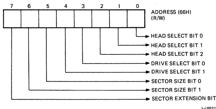
Figure 4-12 SDH Byte Register Format
