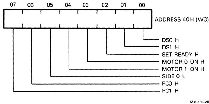
Figure 3-16 Disk Drive Control Register (Z80A) Format
