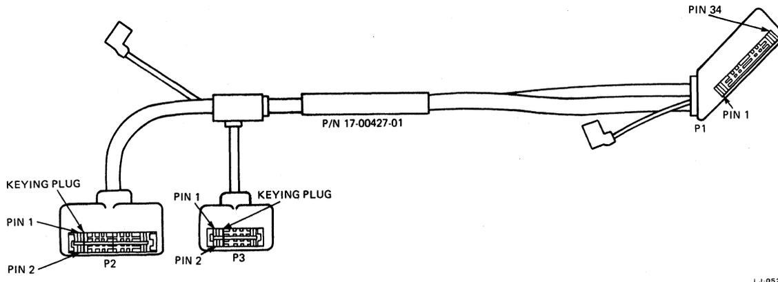
Figure 4-3 Controller/Hard Disk Interconnect Cable
