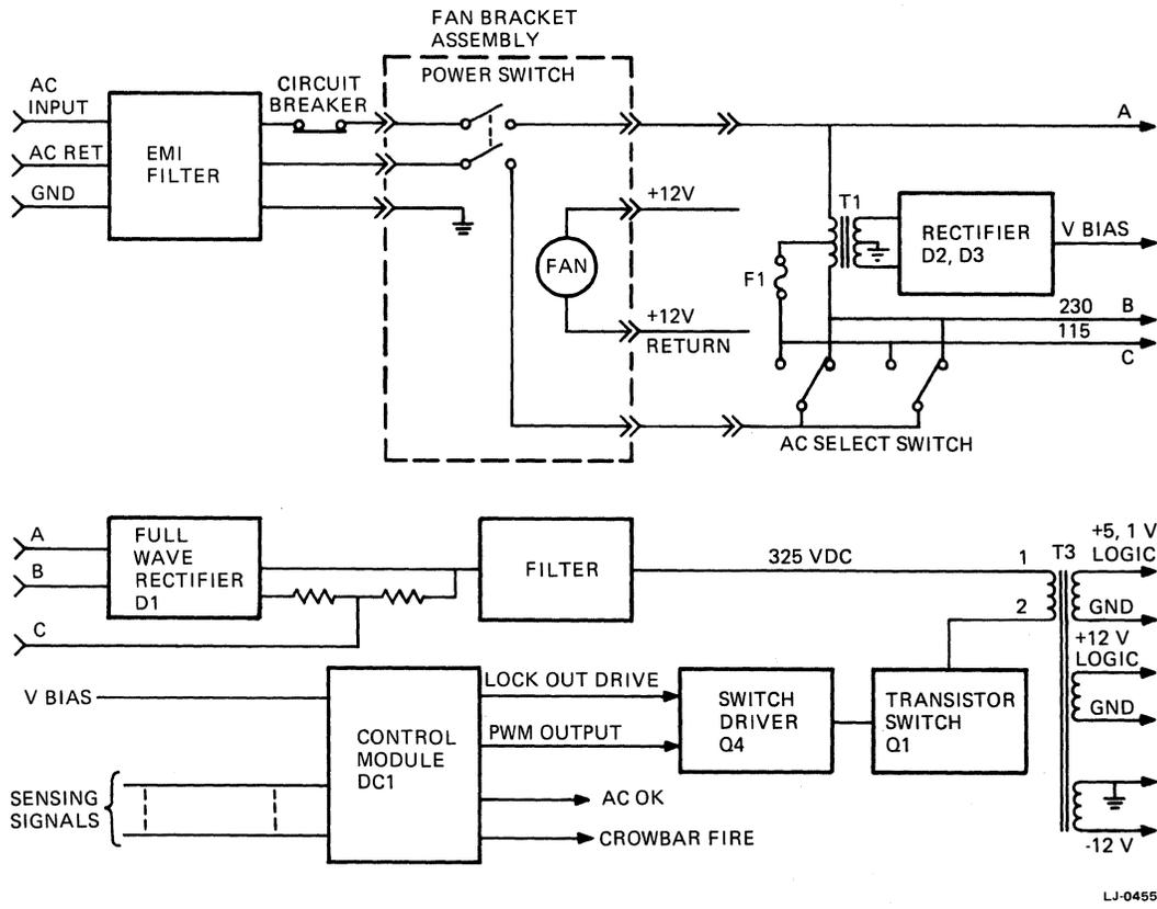
Figure 5-4 Power Supply Functional Diagram
