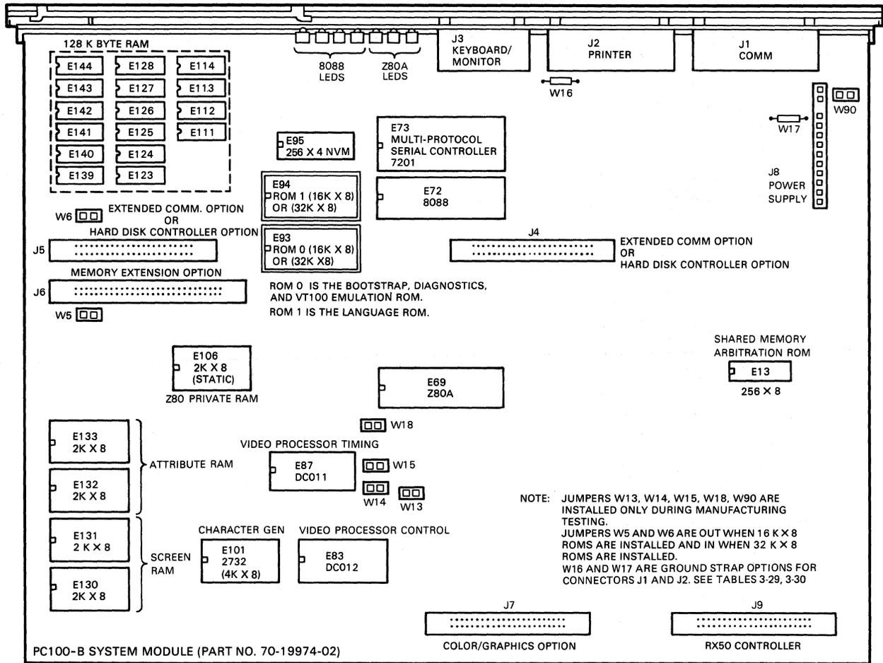
Figure 3-2 PC100-B System Module Physical Layout
