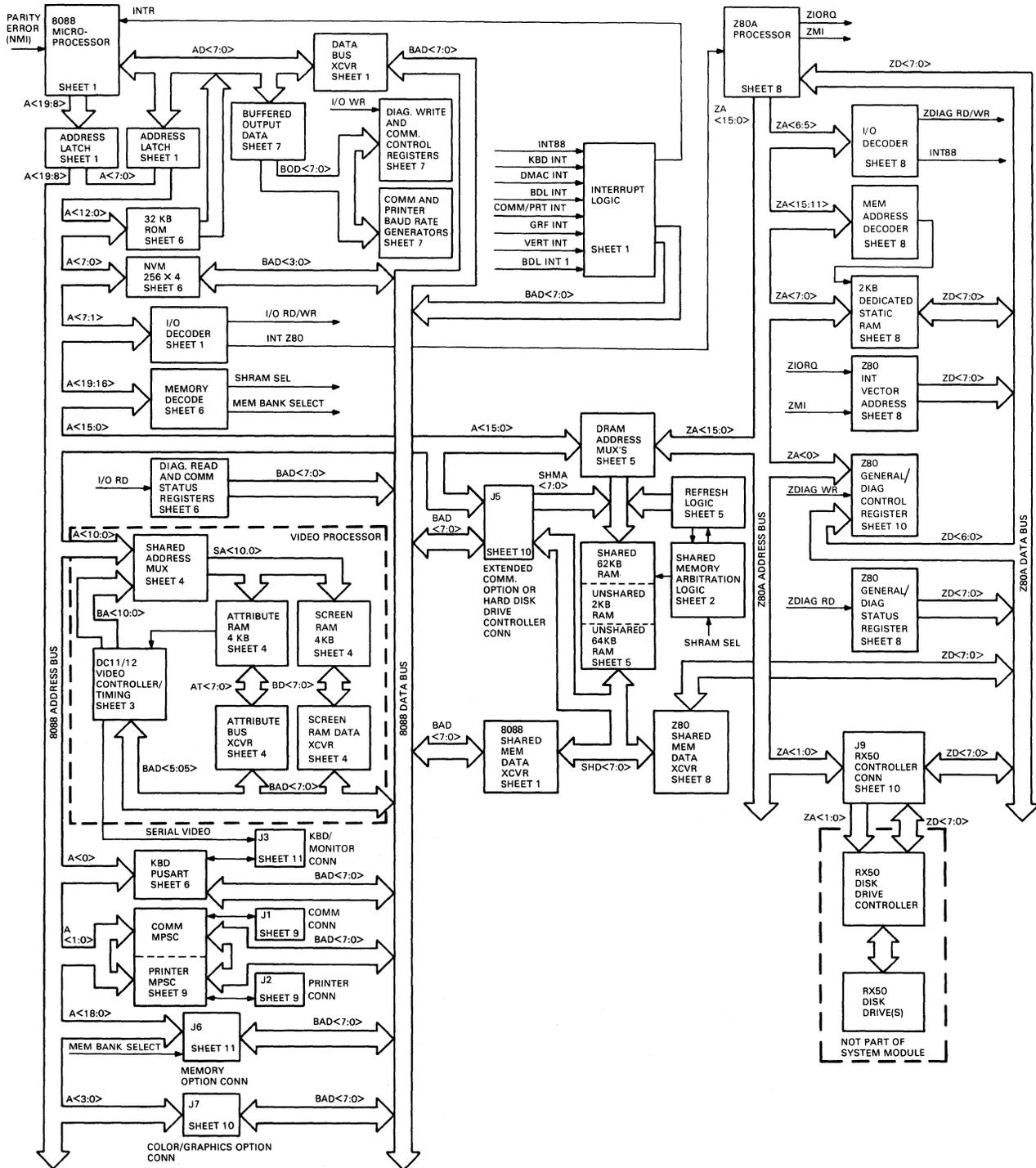
Figure 3-3 PC100-B System Module Address and Data Buses
