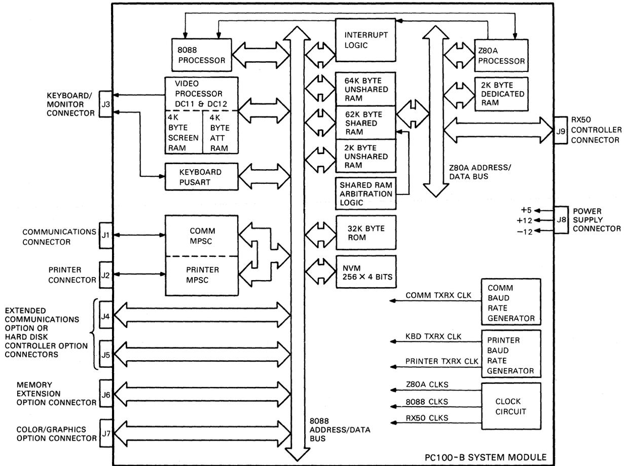
Figure 3-1 PC100-B System Module Block Diagram
