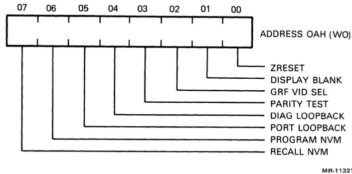
Figure 3-9 Diagnostic Write Register (8088) Format
