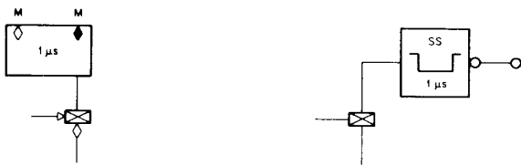
Figure 1-12 Monostable Multivibrator (Single Shot)
