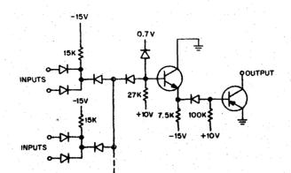
Figure 26 Diode Gate Circuit
