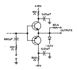
Figure 24 Bus Driver Output Circuit
