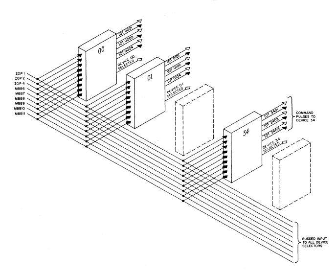
Figure 7 Generation of IOT Command Pulses by Device Selector
