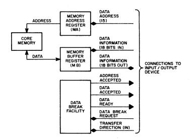
Figure 18 Data Break Transfer Interface Block Diagram
