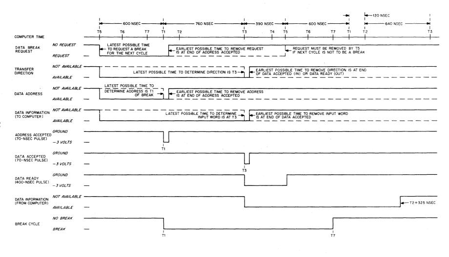
Figure 19 Data Break Transfer Timing Diagram
