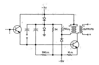
Figure 25 Pulse Amplifier Output Circuit
