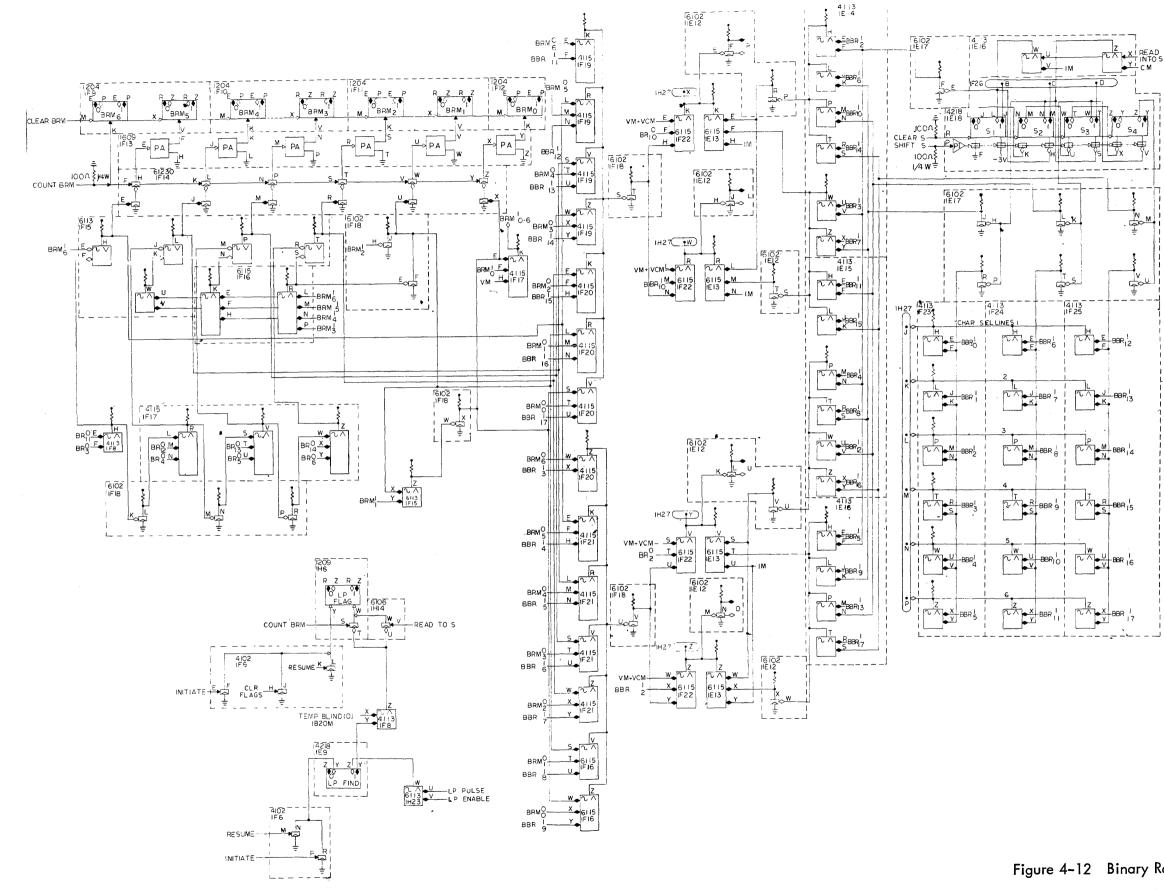
Figure 4–12 Binary Rate Multiplier and Increment Logic BS-E-340-5-20
