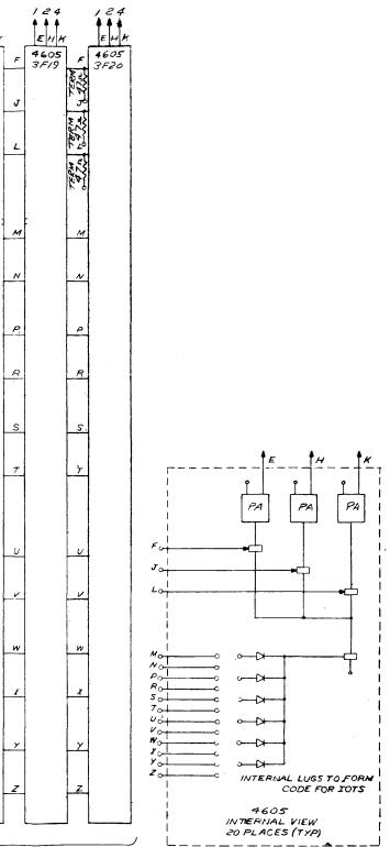
Figure 4-21 Device Selector IOT Decoding BS-D-4C-24-15
