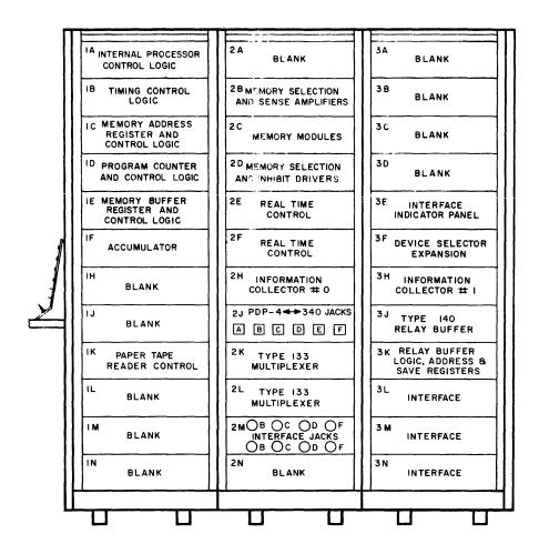
Figure 1-1 PDP-4C-24 Rack Layout
