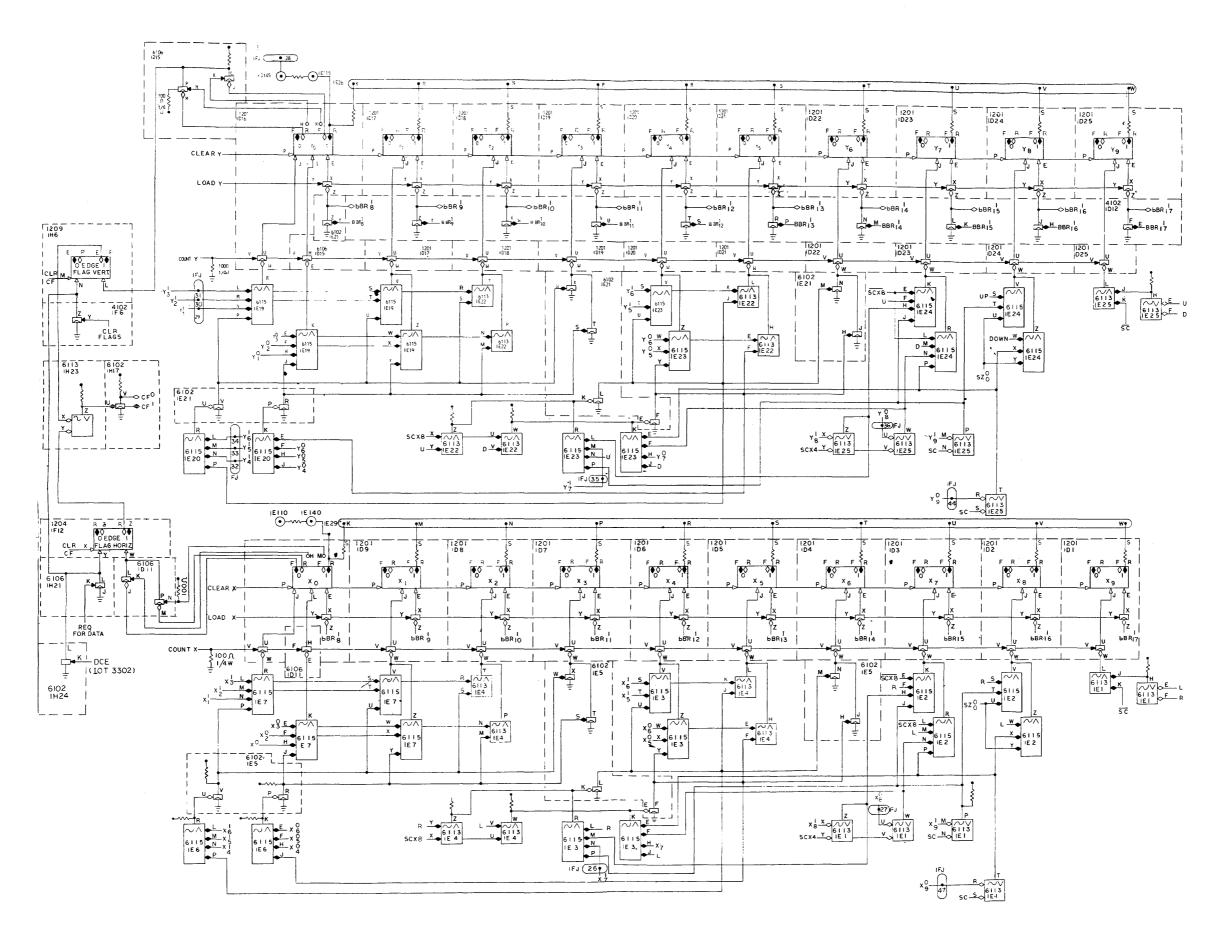
Figure 4–11 Horizontal and Vertical Deflection Registers BS-E-340-5–19
