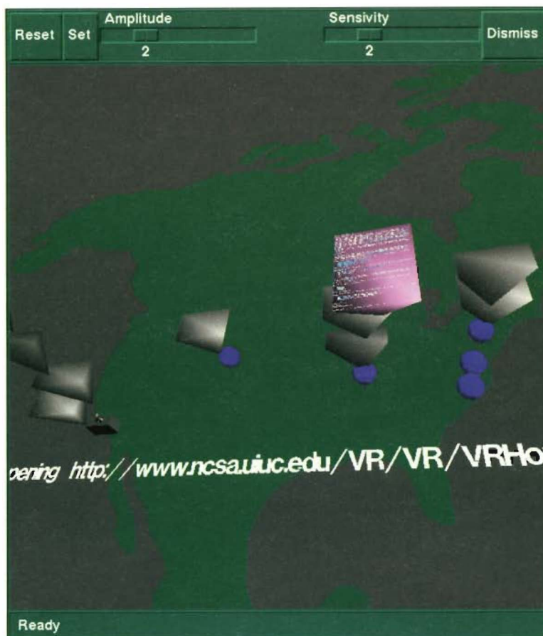
Figure 11 Results of a Tecate Browsing Session Showing a Hyperlink and a Forest of Pyramids That Represents the User's Travels on the Web
