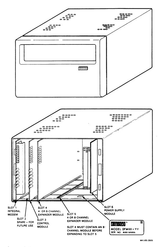
Figure 3-1 DFM Enclosure, Module Placement, and ID Decal
