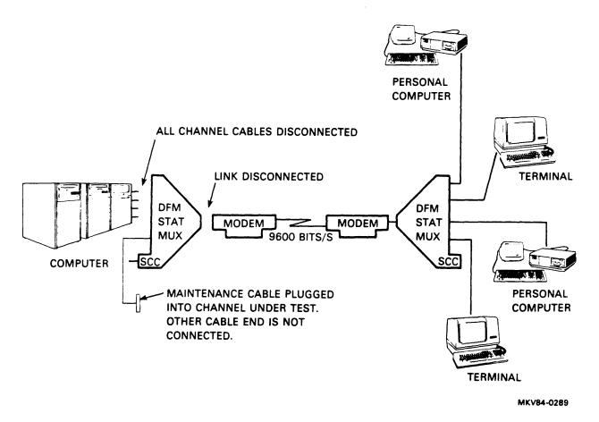
Figure 7-11 Channel Signals Test Configuration
