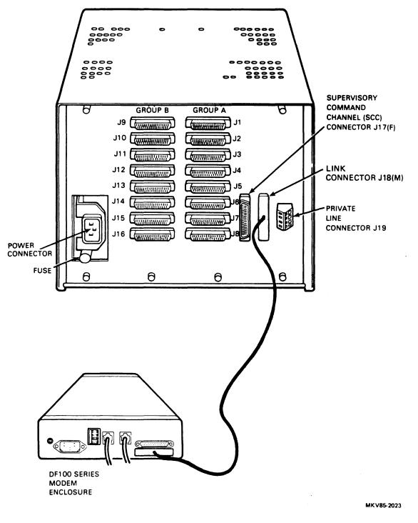
Figure B-1 Standalone Link Modem Connections
