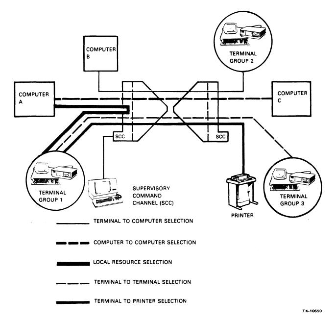
Figure 1-3 Switching and Contention Configuration
