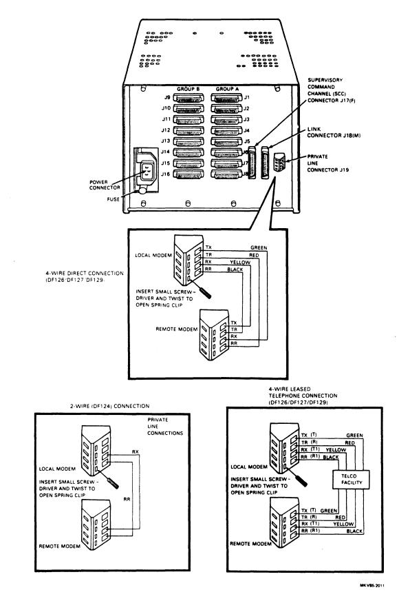
Figure 3-6 Integral Modem Link Connections
