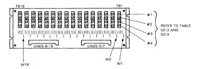
THE APPROPRIATE JUMPERS W1-W16 (ONE FOR EACH LINE) MUST BE INSTALLED IF THAT LINE IS OPERATING BELOW 300 B/S. JUMPER MUST BE REMOVED FOR LINES OPERATING HIGHER THAN 300 B/S
