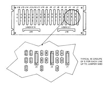
ALL JUMPERS FOR NORMAL CONFIGURATION MUST BE INSTALLED EXCEPT FOR FORCE BUSY (W2, W7, W12, W17, W22, W27, W32, W37, W42, W47, W52, W57, W62, W67, W72 AND W77; THESE JUMPERS MUST BE REMOVED.
