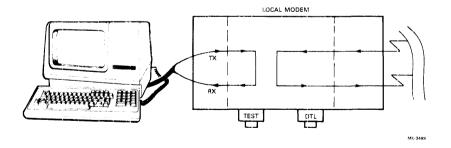
Figure 3 Local-End Digital Loopback Test (DF02 Only)
