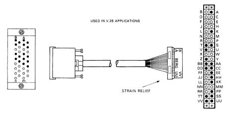
\* INDICATES CAVITIES USED TO MOUNT STRAIN RELIEF
