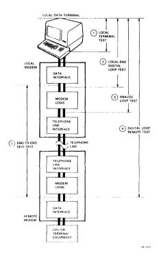
Figure 1 Data Path Acceptance Test Sequence
