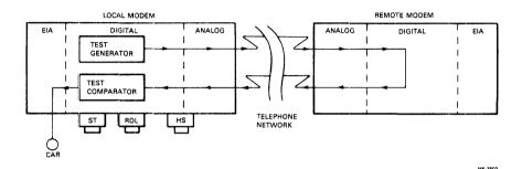
Figure 9 Remote Digital Loopback Self-Test (DF03 Only)
