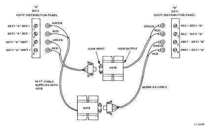
NOTE: THE CABLE ATTACHED TO THE H319 SHOULD HAVE THE CONNECTOR REMOVED AND RING LUGS ATTACHED TO THE RED AND GREEN LEADS AS SHOWN.
