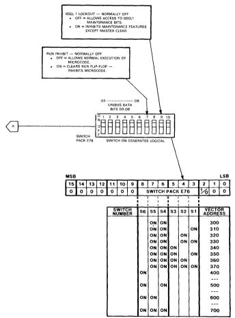
NOTE: SWITCH ON PRODUCES LOGICAL ONE ON THE UNIBUS.
