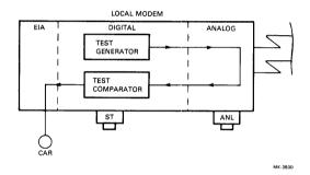
Figure 4 Analog Loopback Self-Test (DF03 Only)
