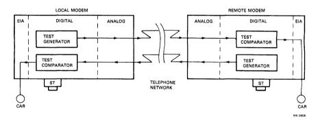
Figure 10 End-to-End Self-Test (DF03 Only)
