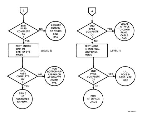
Link Testing Flowchart (Sheet 4 of 4)
