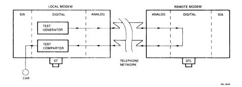
Figure 7 Digital Loopback Self-Test (DF03 Only)
