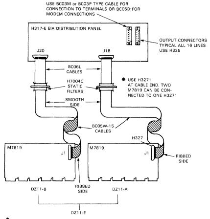
WHEN CONNECTING CABLE TO H3271, BE SURE THAT RIBBED SIDE FACES OUT.
