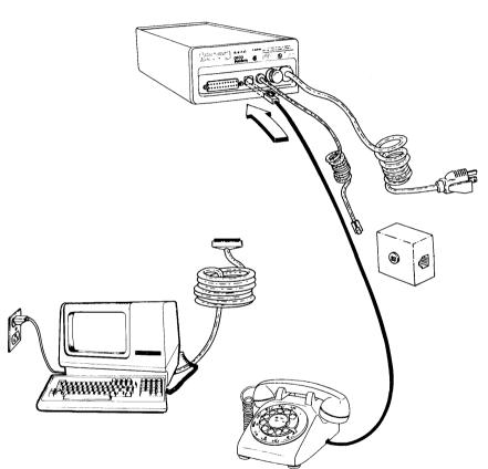
STEP 2. PLUG TELEPHONE INTO JACK ON MODEM.
