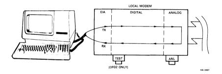
Figure 5 Analog Loopback Test
