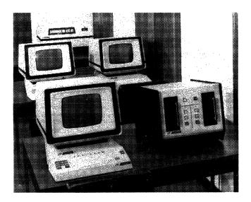
The SPD 20 Family of terminals includes a cluster of display stations such as those shown above. The Terminal Processing Unit (TPU) is in the background; the dual-diskette unit, in the foreground.
