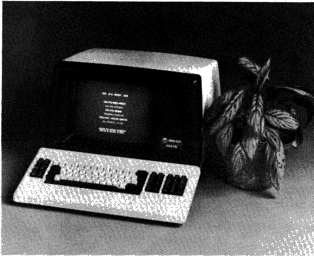
Beehive International's new DM78 display is an ASCII terminal designed to emulate the IBM 3278 display when attached to a protocol converter. Beehive's line of display terminals includes a wide variety of Teletype-compatible models, an IBM 3101 emulator, an IBM 3275/3276 emulator, and a Burroughs TD 830/MT 983 replacement.
