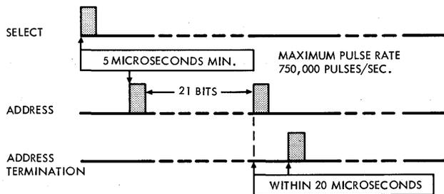
FIGURE XIV TIMING DIAGRAM OF ADDRESS-STATE
