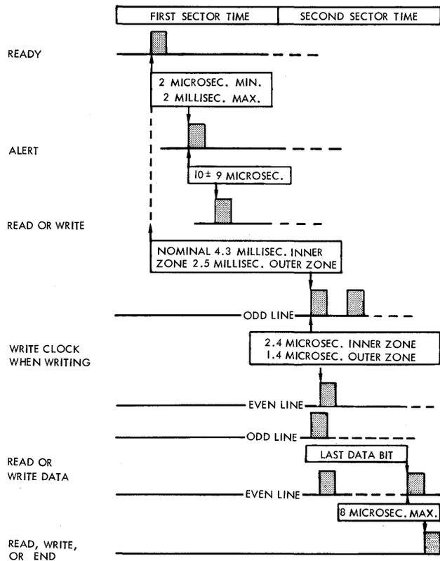
FIGURE XV ACTION-STATE TIMING DIAGRAM
