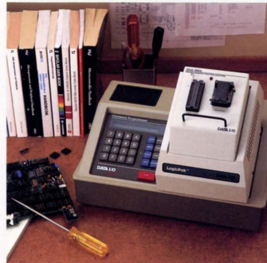
Equipped with the LogicPak<sup>™</sup>, Data I/O's 29B, 29A, or 19 mainframe becomes the sophisticated Programmable Logic Development System (PLDS) for designing, programming and testing virtually every programmable logic device.
