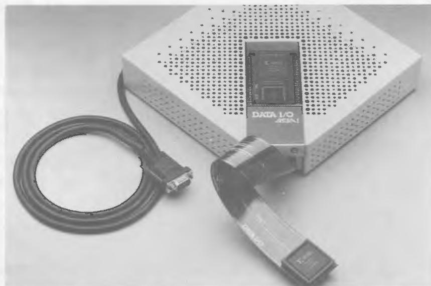
**1. THE MESA I IN-CIRCUIT VERIFIER** facilitates the prototyping, verification, and debugging of programmable gate-array designs. A probe connected to the chassis by a flex-circuit cable plugs into the array's socket in the target system and, in turn, holds the chip being debugged.
