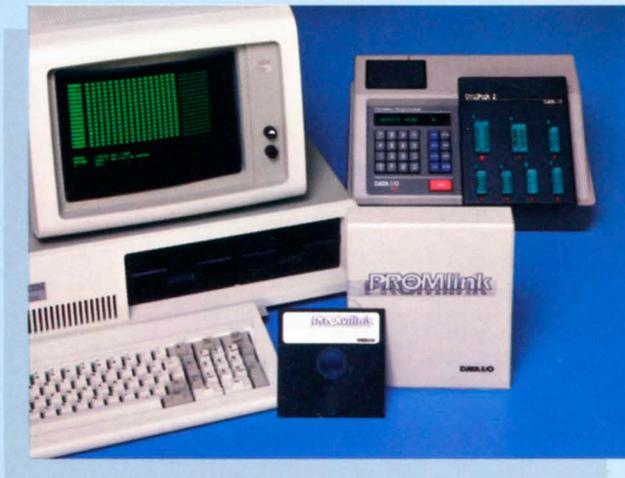
**PROMlink** is Data I/O's software driver that provides a turnkey interface to an IBM-PC so that you control the 29B from the PC. You get the ease of menu-driven commands without the time-consuming hassle of writing your own programs. And PROMlink makes it easy to download data files because it turns your IBM-PC into a highly flexible data storage system.
