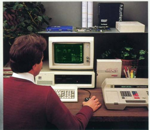
DASH-ABEL allows design engineers to express the design of PLDs in the same schematic form as the entire circuit.
