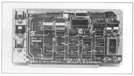
The Model ADC-12 A/D I/O board provides 16 channels of A-to-D conversion with a conversion time of 30 microseconds.
