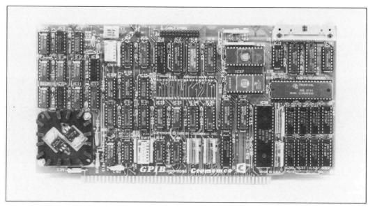
This card enables you to connect your Cromemco computer to measuring and control equipment that has an IEEE-488 port, the communications standard in instrumentation applications. This allows arrangements such as a computer-operated measuring and control system to be devised.
