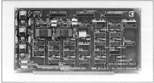
The Model DAC-12 D/A I/O board provides two independent channels of D to A conversion with a conversion time of 5 microseconds.
