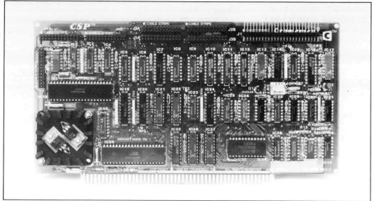
This card interfaces to the C-bus of our I/O Processor card and provides general-purpose I/O capability as well as serial communications capability.
