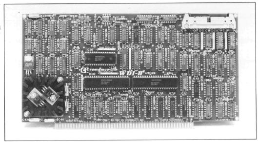
The WDI provides an interface between the system S-100 Bus and a hard disk drive. The WDI circuits, together with the operating system, format and control data transfer between the system main memory and the disk surface media. High speed memory-to-memory data transfers may be made between addressed locations in system main memory. The extended address function allows extended addressing using address-as-data information received from the S-100 bus.
