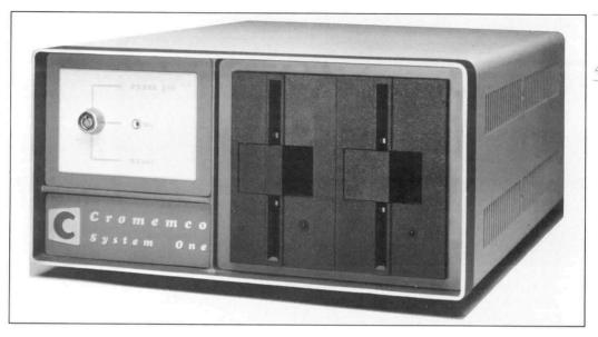
The System One is an 8-slot S-100 bus system which can be used for Z-80A or 68000 system development. The basic System One (Model CS-1) comes with Cromemco's Z-80A processor (ZPU), floppy disk controller (16FDC), and 64K RAM memory (64KZ). The unit has two 5-1/4" floppy disk drives with 780K storage capacity.
