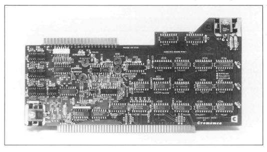
Cromemco's high performance D+7A I/O gives you a way to get analog information into and out of a microcomputer easily, quickly and inexpensively. The Model D+7A offers 7 channels of 8-bit analog-to-digital conversions (to input analog data to the computer); 7 channels of digital-to-analog conversion (to output computer data in analog form); an 8-bit parallel I/O port to input and output data in digital form; and a fast conversion time of 5.5 microseconds.
