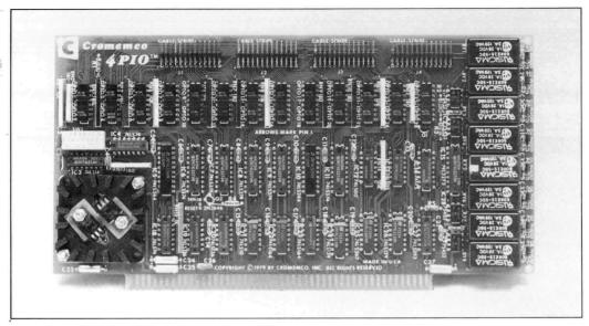
The Cromemco 4PIO Parallel Interface Card allows interfacing with complete electrical isolation from the host microcomputer. Therefore, problems with ground noise and ground loops can be completely eliminated in instrumentation, communications, or process control systems. In addition, potentially damaging transients can be safely isolated from the computer system.
