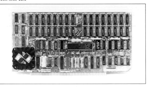
Cromemco's 256KZ RAM card is an S-100 bus compatible 256K byte read/write memory board. This board is ideal for use with Cromemco's CROMIX multi-user, multi-tasking operating system.
