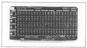
For use with the DPU, Cromemco offers a 512 kilobyte RAM memory unit. This unit works under the control of a new Memory Controller Unit (MCU) which supports either byte or word-width operation.
