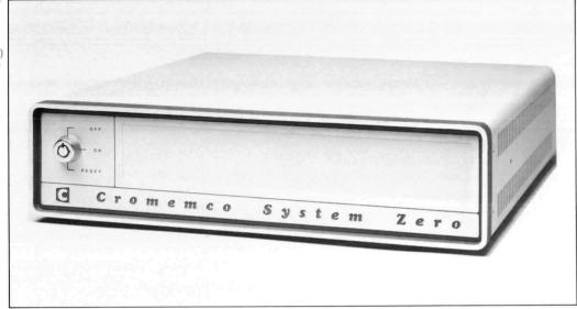
The System Zero (Model CS-0) is designed for development of systems based on Cromemco's Single Card Computer (Model SCC). The CS-0 has four S-100 slots, one of which is occupied by the SCC. Cromemco's Monitor and Control Basic firmware (MCB-216) is included.
