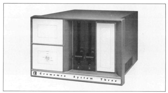
The top-of-the-line System Three (Model CS-3A) uses 8-inch floppy disk drives (1.2 Megabyte capacity each) and has 21 S-100 card slots. The hard disk version (Model CS-3H) replaces one of the 8-inch floppy drives with a 21 Megabyte Winchester hard disk drive.
