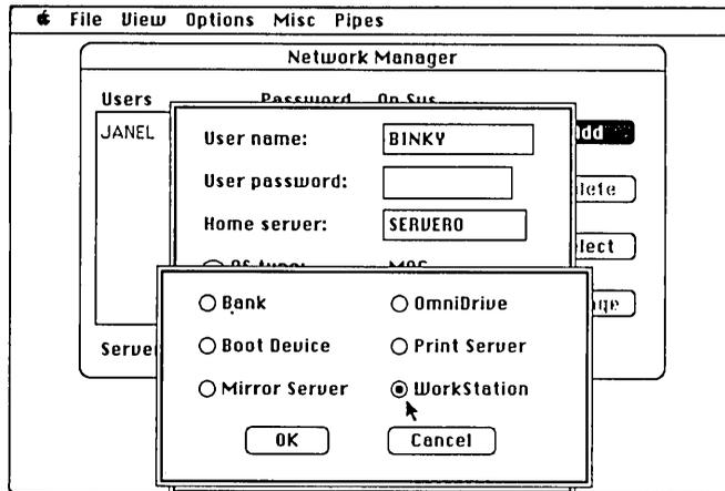
Click OK to return to the previous menu, then type in the Omninet address of the Macintosh that will perform the device boot. If you do not know the address, compare the setting of the address switches on the Macintosh's Transporter box with the network address chart in Chapter 3 of this guide. When you have entered the information, click OK.
