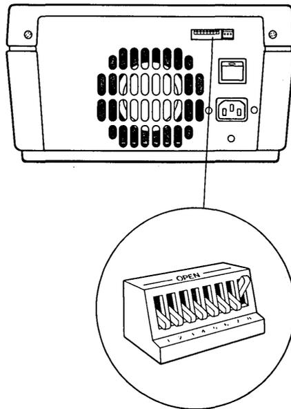
Switches 7 and 8 are not used for setting the device address. Switch 7 should be pushed toward the numbers for ALL OmniDrives. Switch 8 is the bias switch. Only one OmniDrive on a network should have the bias switch pushed toward the numbers.
