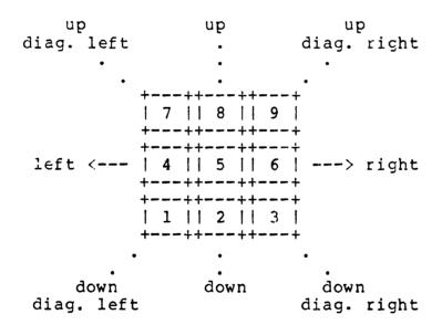
The cursor keys move the picture in smaller increments for fine tuning. The cursor keys allow you move the picture left, right, up and down.
