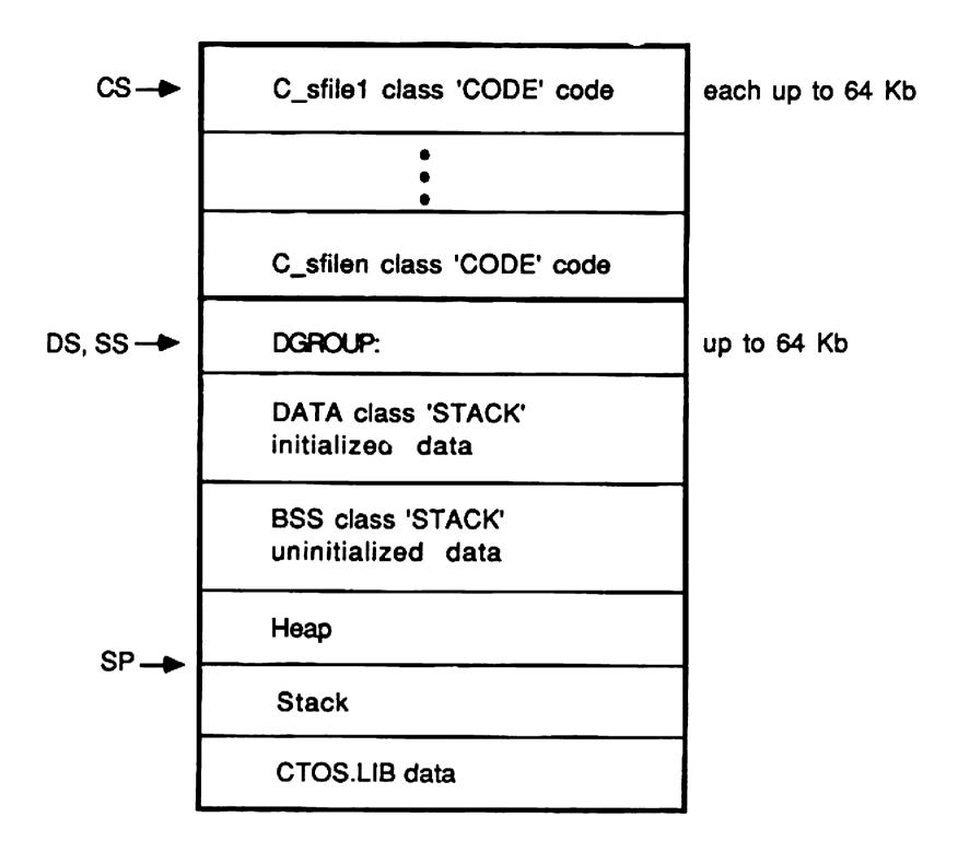
In the large and huge models, the stack is located independently of the heap, and grows downward towards the start of the data segments. Note that the first data segment still combines CTOS.LIB data with the stack. In these models the heap can extend to fill all of short-lived memory.
