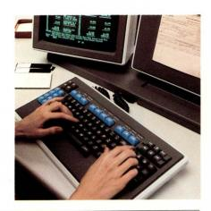
The keyboard is also elevated and angled so your operator can work for longer periods without becoming tired.
