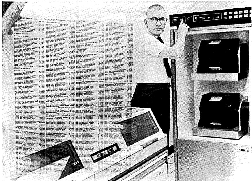
— Computer-based Phototypesetting: It takes this new IBM photocomposing unit less than eight seconds to typeset a full page for a telephone directory. Controlled by an IBM System/360 computer, it can set a newspaper page in ten seconds and a full-length novel in about ten minutes.
