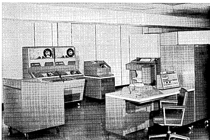
EAI 640 DIGITAL SYSTEM / Electronic Associates, Inc. — EAI's second purely digital system offers the input-output flexibility and software for use both as a stand-alone system and for integration into hybrid and special computer-based systems. Options include expansions for teletype equipment, a direct memory-access channel, and memory expansions from the basic 4K words to 8K, 16K or 32K. The 640/610 Line Printer (right rear in system photo) is shown at the right with cover lifted. (For more information, designate #51 on the Readers Service Card.)
