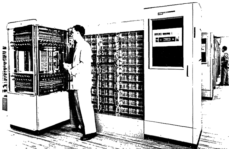
Figure 4 — Power Module on Right. Memory Frame in Center. Memory Array Frame on Left. The heart of the AN/FSQ-7 air defense computer is the magnetic core memory. This memory contains over 500,000 bits of high-speed storage with an access time of six millionths of a second to any group of 32 bits. It will contain the instructions that the computer will follow during its normal operation and the data which is being correlated and processed at that time.
