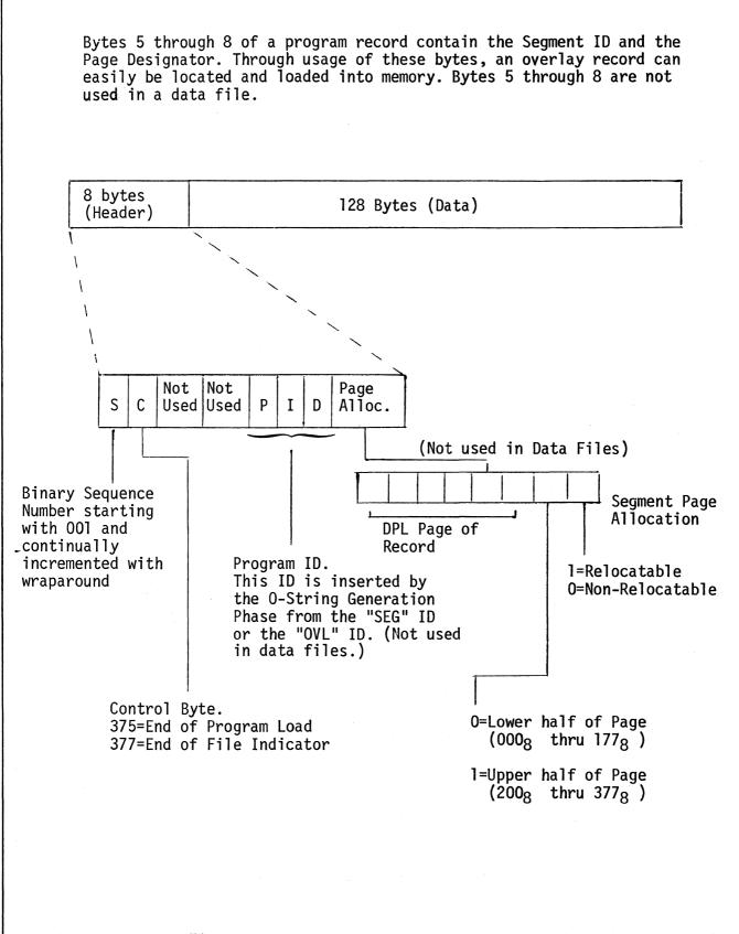
Figure 4. Standard Mini-Tape Record Layout.
