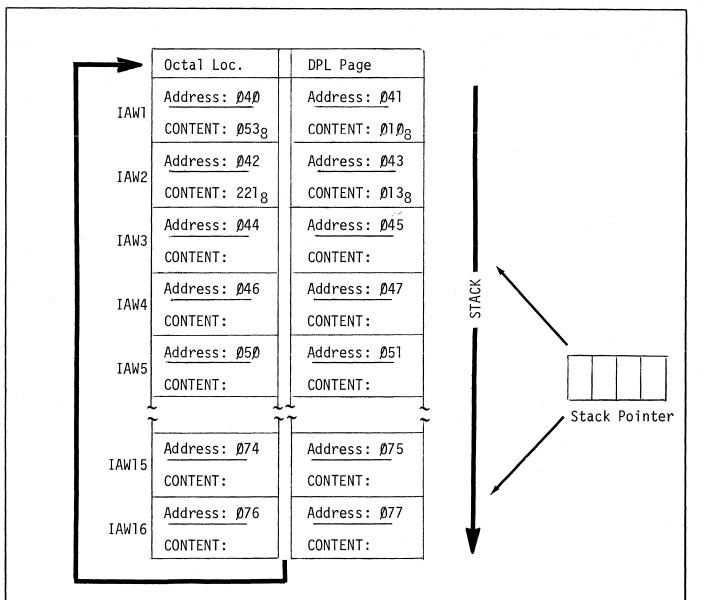
Figure 2. Snapshot of Instruction Address Stack after completion of EXU Instruction (See Example).
