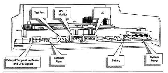
Figure 1-2: Back panel connectors
