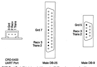
**CMD Test Port:** This is intended for use by CMD service personnel and has no application during normal operation of the controller.
