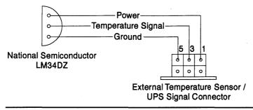
Figure 1-4: External temperature sensor wiring diagram
