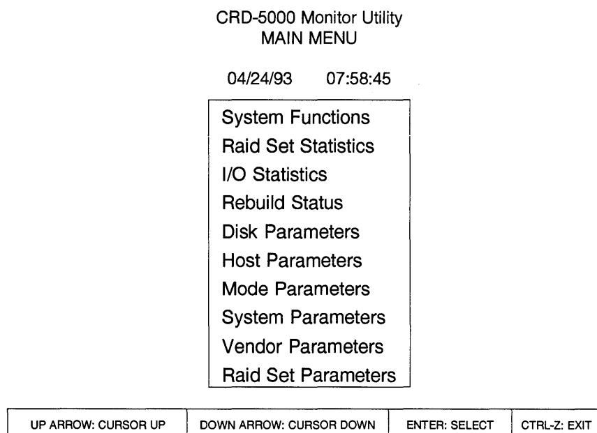
This screen is identical to the user-level main menu, except for the additional options "Mode Parameters" and "Vendor Parameters."
