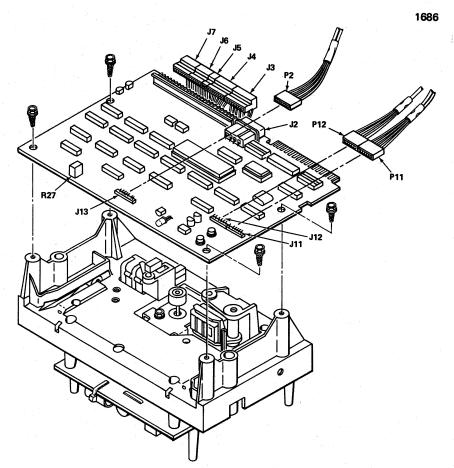
Figure 3-6. Main PWB Removal
