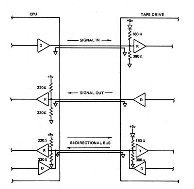
Figure 2-4. Line Driver/Receiver Terminations
