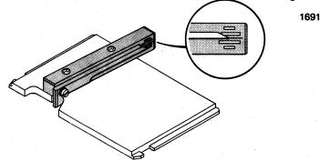
Figure 3-11. Zenith Alignment Tool
