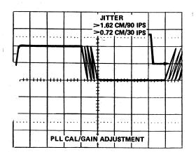
Figure 3-25. Phase Lock Loop Adjustment incrementing and reset to zero. Tape motion should then reverse until file mark on tape is repositioned under head. Tape should then start forward and second 400-block file should be written and block counter should start
