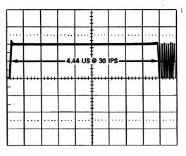
Figure 3-23. Gap Adjustment Display Pattern
