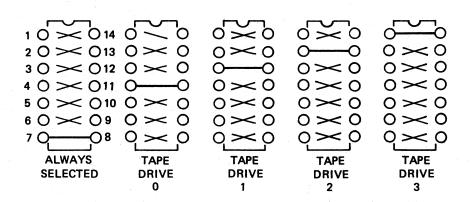
Figure 2-8. Multiple Tape Drive Address Shunt
