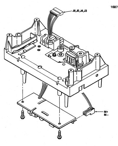
Figure 3-7. Motor Driver PWB Removal
