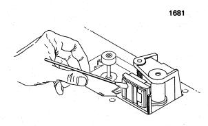
Figure 3-2. Head Assembly and Tape Cleaner Cleaning
