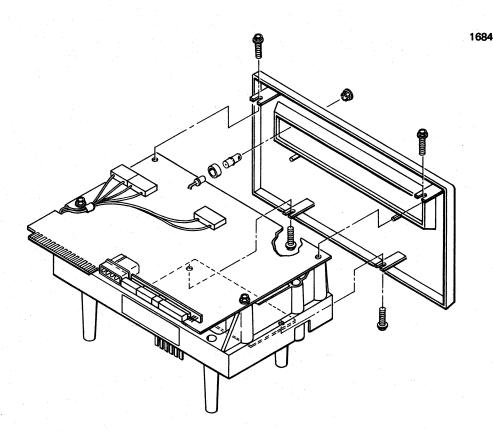
Figure 3-4. Front Panel Removal
