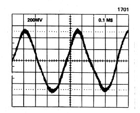
on BE101 from position 1 to Figure 3-22. Read Circuit Output Voltage position 2 and record observed peak-to-peak voltage.
