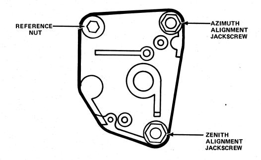
Figure 3-12. Jackscrew Locations on Head Carriage Assembly
