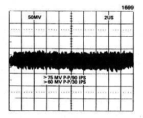
Figure 3-20. Erase Residue Voltage
