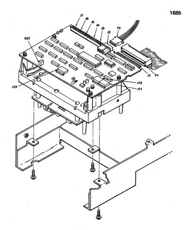
Figure 3-5. Basic Tape Drive Removal
