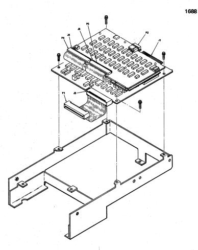
Figure 3-8. Formatter/Controller PWB Removal
