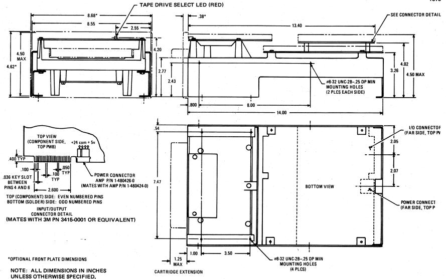
Figure 2-3. Quarterback Tape Drive Mounting Dimensions
