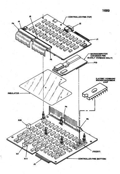
Figure 3-9. Microcomputer Expander PWB Removal
