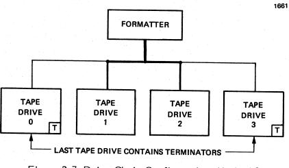
Figure 2-7. Daisy-Chain Configuration, Method 2
