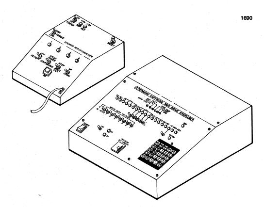
Figure 3-10. BE101 and SME Control/Indicator Panels
